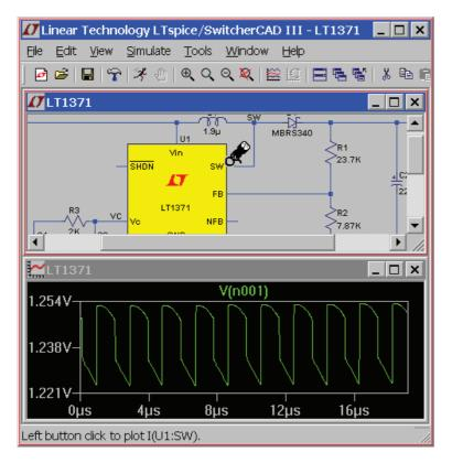
When plotting a pin current, the convention of positive current is in the direction into the pin.
