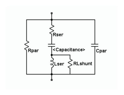
Capacitor Instance Parameters
