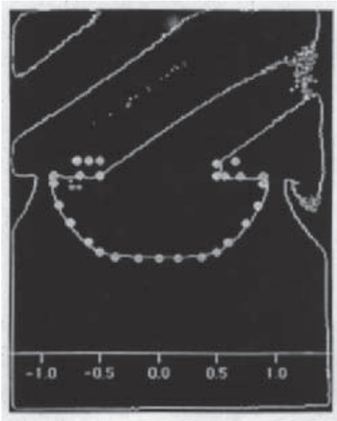
Figure 9. The digitized profile of the trench etched for 1.5 minutes. The simulation is shown superposed on the digitized image.
