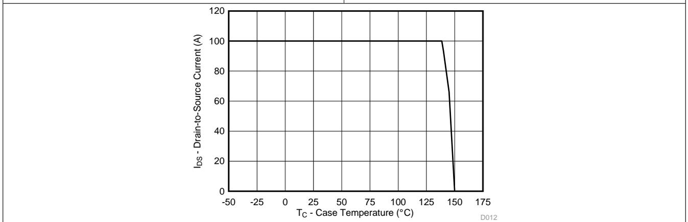
Figure 12. Maximum Drain Current vs Temperature
