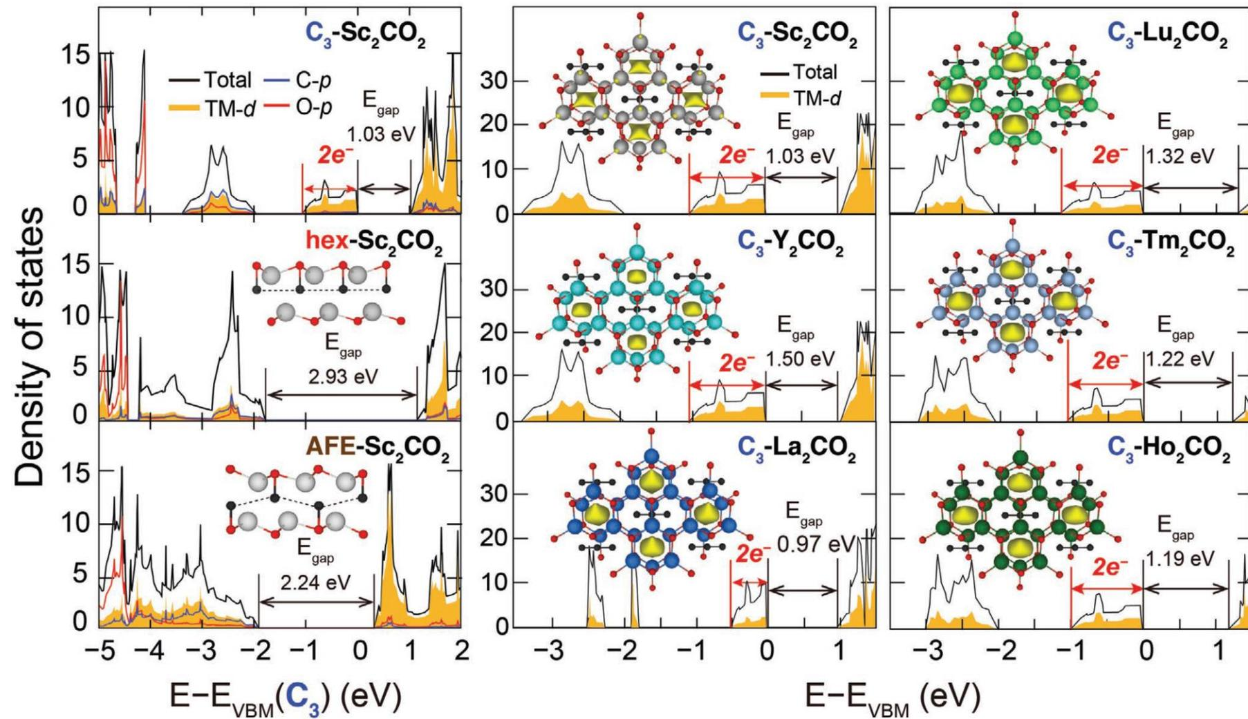
**Figure 3.** Density of states of  $C_3-M_2CO_2$  ( $M = Sc, Y, La, Lu, Tm$  and  $Ho$ ) and  $Sc_2CO_2$  in hex and AFE phase and partial charge density of in-gap states. The band gap is denoted with arrows. The zero of energy is set to the valence band maximum (VBM) of  $C_3-M_2CO_2$ . The isosurface of the partial charge density plots is set to  $0.01e$  per bohr<sup>3</sup>.
