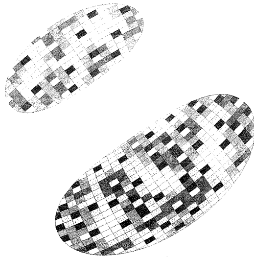
5.7: Panel Type Distribution on Canopies. Source: Brady Peters, based on Foster + Partners design
