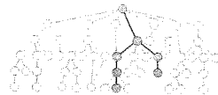
9.3: The explicit space (in orange) expresses the path(s) taken by a designer to reach a solution. It is a subgraph of the implicit space (in grey).
