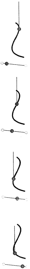
8.2: A simple CONTROLLER. The point on the line controls the point on the curve, which, in turn, is the base for a vertical line.
