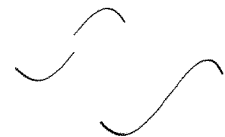
7.16: A split function creates a gap right in the middle of the S-curve, which is then connected with a linear member. Source: Onur Yüce Gün and KPF.
