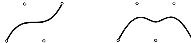
6.89: An order 4 curve with five points on its control polygon allows a single "dip". This simple and computationally light description is sufficient for many design situations.
