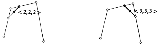
6.75: The level 2 control points for \langle 2, 2, 2 \rangle (on the left) and \langle 3, 3, 3 \rangle (on the right). Each has its respective blossom values as computed by the second level of the deBoor algorithm. The level 3 points are already computed at this stage as one of the level 2 control points.
