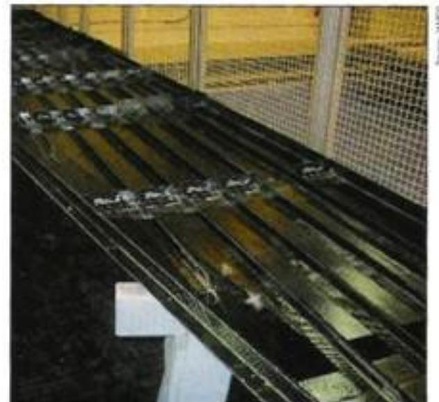
JAMCO's pultruded carbon fiber/epoxy stringers are shown here after assembly with skin panels for an Airbus vertical tail.
