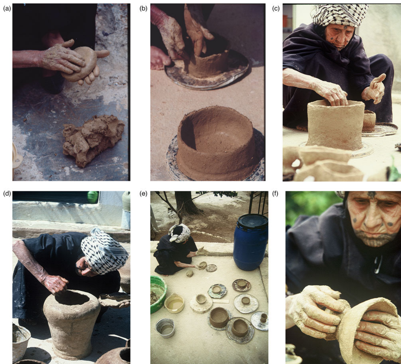
Fig. 12.6 Views of a traditional potter making coil-built vessels in a village in northern Jordan in 1995 (photos by E. Grossmith): (a) forming a disk base, (b) the lower parts of two vessels, (c) building up the walls
