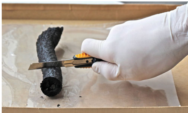
Fig. 16.11 Fracturing a charred branch fragment in the transverse plane by gentle pressure with a sharp scalpel
