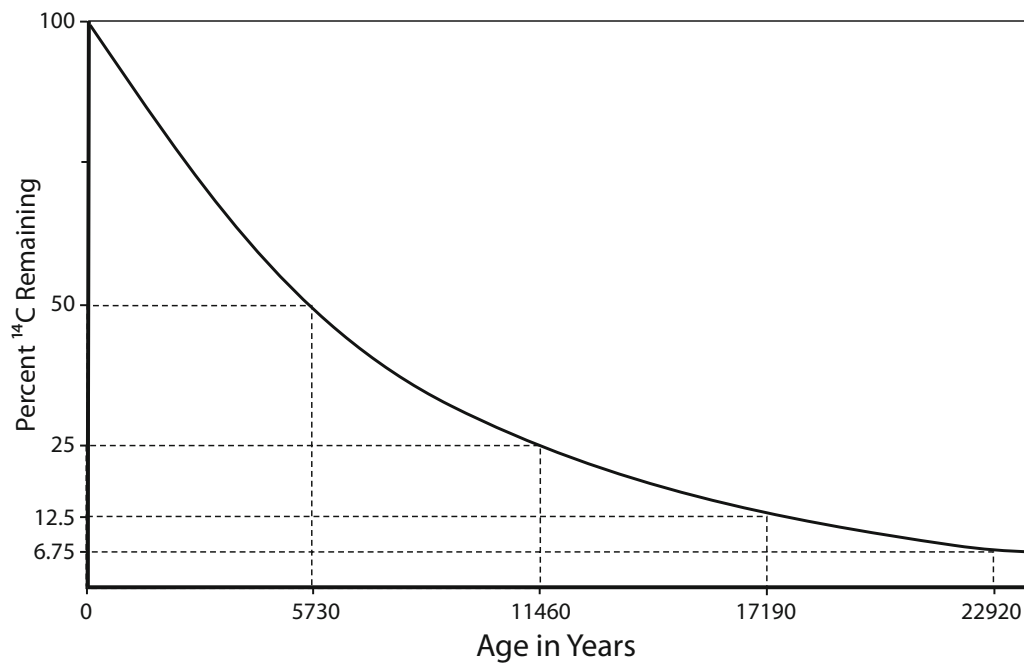
Fig. 20.8 Exponential decay of ^{14}\text{C}
