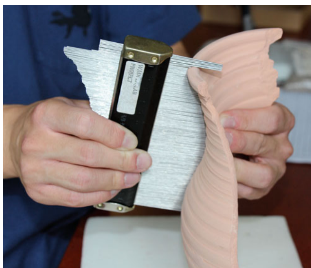
Fig. 21.6 Use of a profile gauge to reproduce complex shapes
