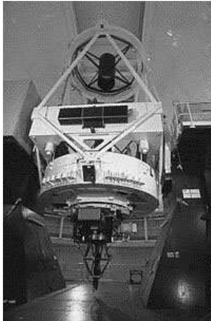
Figure 16.29. The William Herschel Telescope (WHT)—4.2 m. This telescope is driven on an alt-azimuth mounting. (Photograph by courtesy of the ING of Telescopes, La Palma.)
