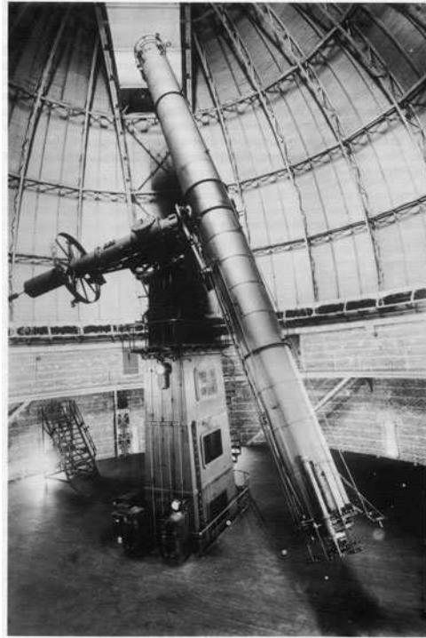
Figure 16.27. The 40-inch Yerkes refractor. (By courtesy of the Royal Astronomical Society.)
