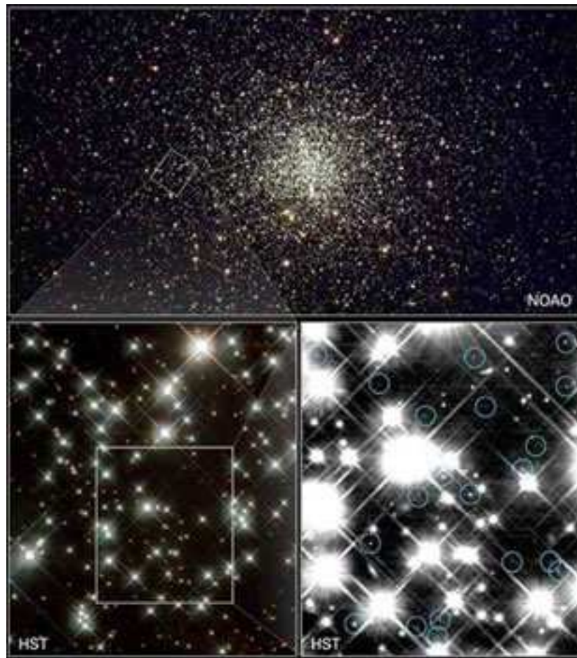
Figure 17.3. The upper frame is by a ground-based telescope of a star field. A section of this has been observed by the HST telescope. The lower right frame is further magnified and, without the effects of atmospheric seeing, clearly shows the telescope diffraction pattern imposed on the brighter stellar images. The circles indicate the positions of very faint stars. (By courtesy of STScI.)
