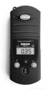
**FIGURE 13-17** Photograph of a simple LED-based colorimeter. (Hach Company, USA.)
