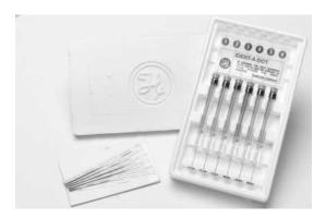
FIGURE 27-3 A set of microsyringes for sample injection. (Courtesy Hamilton Company.)
