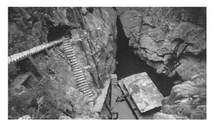
Hongshui River Fengcong Karst, China: A concrete boat, housing pumps for water abstraction, floats in a flooded karst window within the rugged karst terrain of the Disu catchment. (Photo by Tim Fogg)
