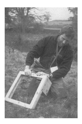
Radiolocation: Figure 3. Using a nulling technique to measure field angle—note the clinometer attached to the side of the receiver loop antenna. (Photo by Mike Bedford)
