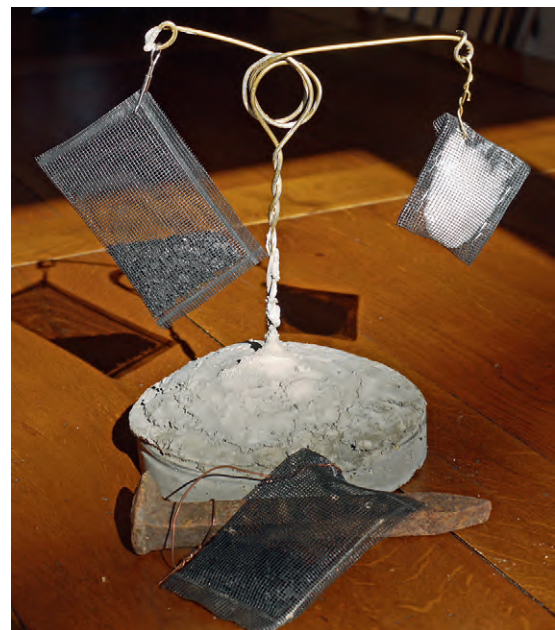
FIGURE 2 A “Quinlan Gumdrop” anchor for passive dye collectors. The base is concrete molded in a coffee can and the detectors are suspended above the bottom of deeper springs or streams. The screen envelopes contain unbleached cotton (right arm) and activated carbon (left arm and bottom). The packets can also be secured with wire to rocks or other solid anchors such as old railroad spikes.
