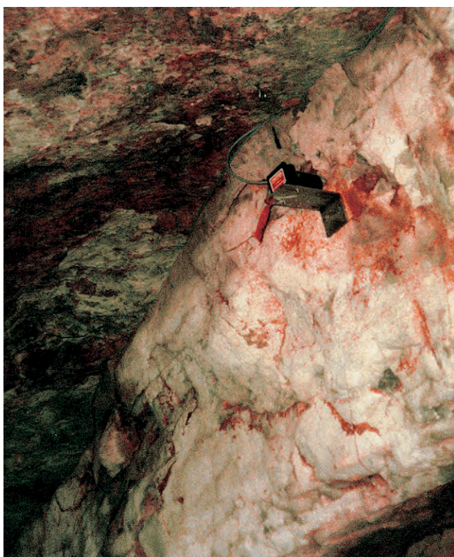
FIGURE 2 Kartchner Caverns (AZ, U.S.A.). Sometime in a cave there are joints which may imply possible rock fall. In order to assure the safest condition in a show cave, it is necessary to detect well in advance any minor movement. A detector, monitoring possible displacement of a limestone layer, can be seen in this photo. Photograph taken by the author.
