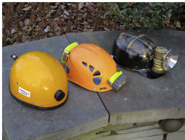
FIGURE 1 A comparison of caving helmets. Left: a rock-climbing helmet fitted with a lamp bracket. Middle: a modern caving helmet with attached LED headlamp and battery pack on the back. Right: a miner's helmet with carbide lamp.
