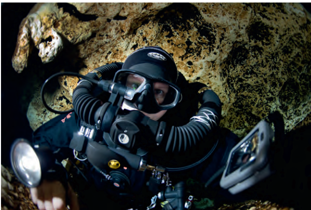
FIGURE 5 The author diving in a Sentinel Expedition rebreather, which offers not only a gaseous carbon dioxide monitor, but also a large heads-up display with lights and vibrating buzzer that alerts the diver to life-threatening scenarios. Photo by the author.
