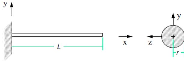
$L = 3.0 \text{ m}$        $r = 0.014 \text{ m}$        $J = 6.0\text{E-}8 \text{ m}^4$
