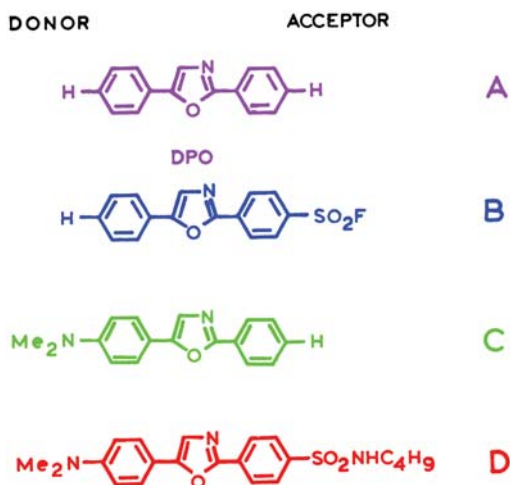
Figure 6.46. Derivatives of 2,5-diphenyloxazole (DPO, A) with donor and acceptor groups (B–D). Revised from [101].
