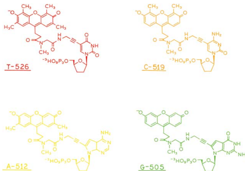
Figure 21.5. Fluorescent chain-terminating dideoxynucleotides. The letters refer to the DNA base, and the numbers refer to the emission maximum. Reprinted with permission from Prober JM, Trainor GL, Dam RJ, Hobbs FW, Robertson CW, Zagursky RJ, Cocuzza AJ, Jensen MA, Baumeister K. 1987. A system for rapid DNA sequencing with fluorescent chain-terminating dideoxynucleotides. Science 238 :336–343 [9]. Copyright © 1987, American Association for the Advancement of Science.
