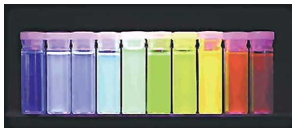
Figure 21.47. Real-color photograph of ZnS-capped CdSe quantum dots excited with a near-UV lamp. From [148].
