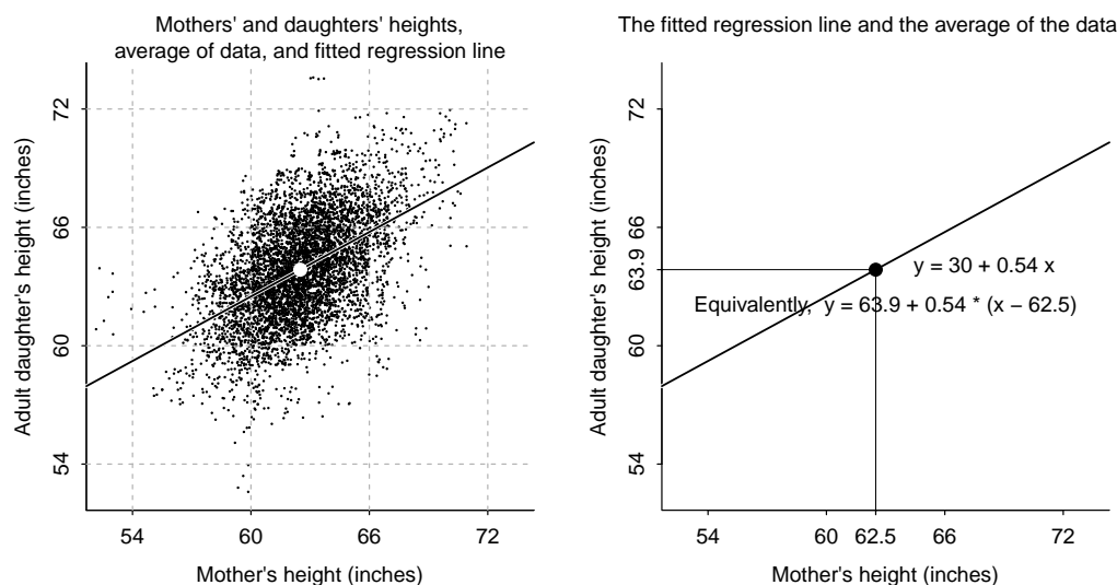
Figure 6.3 (a) Scatterplot adapted from data from Pearson and Lee (1903) of the heights of mothers and their adult daughters, along with the regression line predicting daughters' from mothers' heights. (b) The regression line by itself, just to make the pattern easier to see. The line automatically goes through the mean of the data, and it has a slope of 0.54, implying that, on average, the difference of a daughter's height from the average (mean) of women's heights is only about half the difference of her mother's height from the average.
