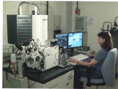
Figure 9–49 The scanning electron microscope. In a SEM, the specimen is scanned by a beam of electrons brought to a focus on the specimen by the electromagnetic coils that act as lenses. The detector measures the quantity of electrons scattered or emitted as the beam bombards each successive point on the surface of the specimen and controls the intensity of successive points in an image built up on a video screen. The SEM creates striking images of three-dimensional objects with great depth of focus and a resolution between 3 nm and 20 nm depending on the instrument. (Photograph courtesy of Andrew Davies.)
