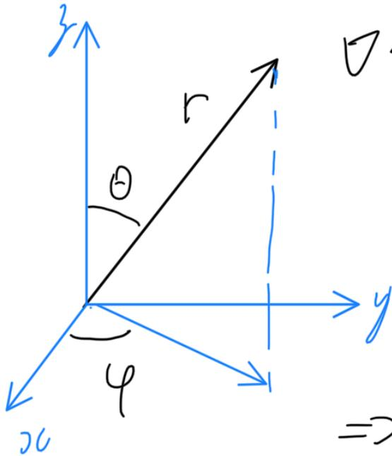
$$\nabla^2 = \frac{1}{r} \frac{\partial^2}{\partial r^2} (r) + \frac{1}{r^2 \sin \theta} \frac{\partial}{\partial \theta} \left( \sin \theta \frac{\partial}{\partial \theta} \right) + \frac{1}{r^2 \sin^2 \theta} \frac{\partial^2}{\partial \varphi^2}$$
