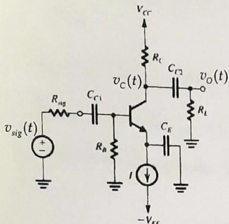
$$V_{CC} = -V_{EE} = 10,0V$$
