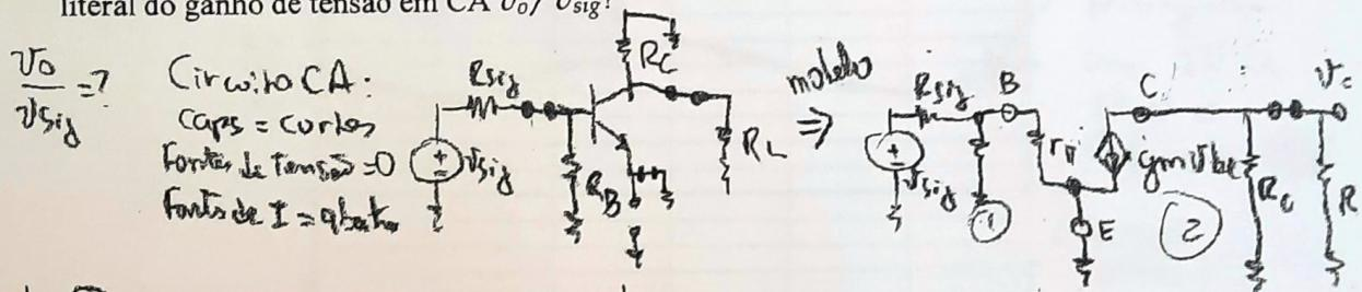
$$\left. \begin{aligned} \frac{v_o}{v_{sig}} &= ? \\ \text{Circuito CA:} \\ \text{caps = curtos} \\ \text{Fonte de Tensão = 0} \\ \text{Fonte de I = geração} \end{aligned} \right\} \text{de (2)} \quad v_o(+) = -(R_C // R_L) g_m v_{be} \\ \left. \begin{aligned} v_{be} &= v_{sig} \frac{r_\pi // R_B}{R_{sig} + R_B // r_\pi} \end{aligned} \right\} \text{de (1)} \quad v_o(+) = -(R_C // R_L) g_m \cdot \frac{r_\pi // R_B}{R_{sig} + R_B // r_\pi} \cdot v_{sig}(+)$$
