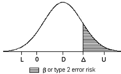
Fig. 4. Illustration of the type 2 error risk \beta in an RCT showing a difference D in effect, which is not significant, since zero (0) difference lies between the lower (L) and upper (U) 95% confidence limits. The type 2 error risk of having overlooked an effect of \Delta is substantial.
