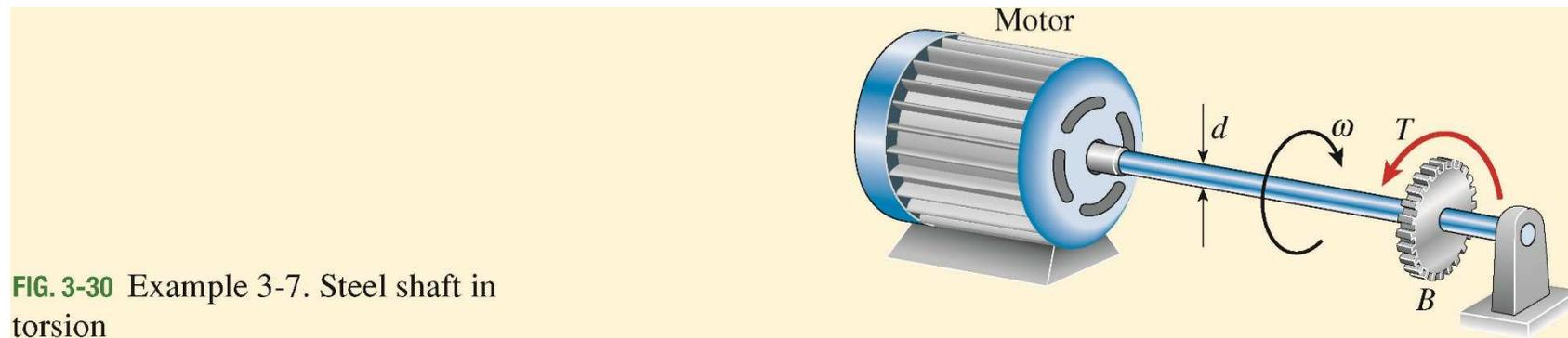
**FIG. 3-30** Example 3-7. Steel shaft in torsion
