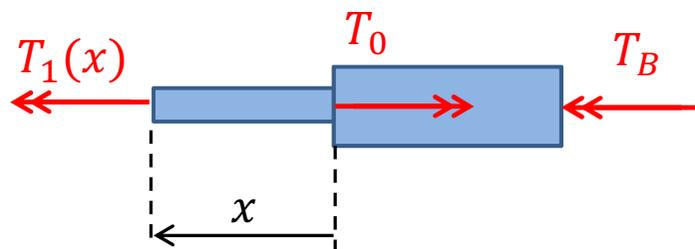
$$T_1(x) + T_B = T_0 \Leftrightarrow T_1(x) = T_0 - T_B \quad (0 \leq x < L_A)$$
