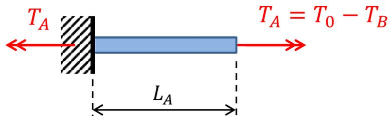
$$\phi_{C,A} = \frac{T_A L_A}{G I_{pA}} = \frac{T_A}{k_{tA}} = \frac{T_0}{k_{tA} + k_{tB}}$$
