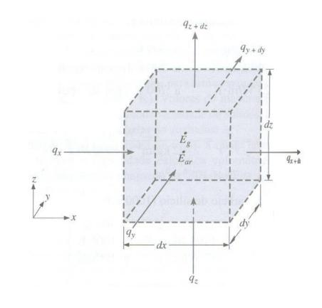
$$\left| \frac{\partial}{\partial x} \left[ k_x \frac{\partial T}{\partial x} \right] + \frac{\partial}{\partial Y} \left[ k_y \frac{\partial T}{\partial y} \right] + \frac{\partial}{\partial Z} \left[ k_z \frac{\partial T}{\partial z} \right] + q_G^{\prime\prime\prime} = \rho C \frac{\partial T}{\partial t}$$
