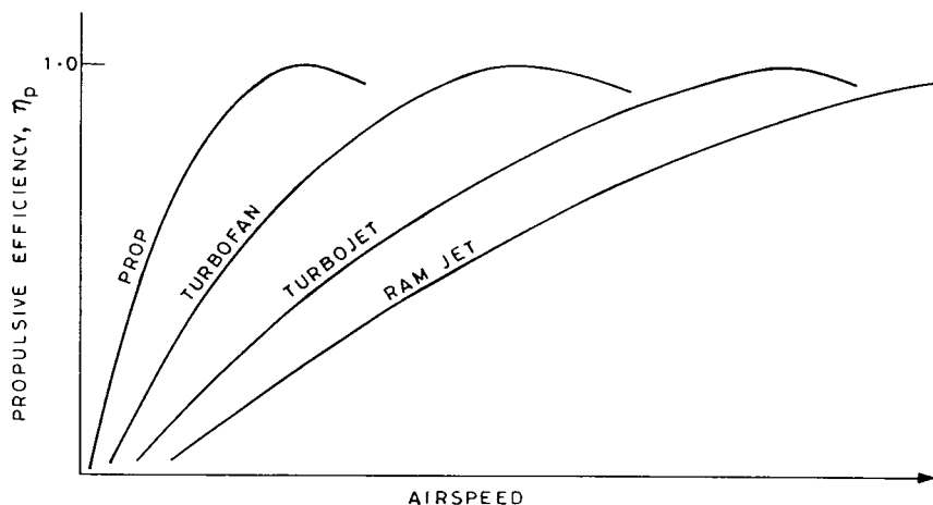
Fig. 4.11 Propulsive efficiency of different airbreathing engines.
