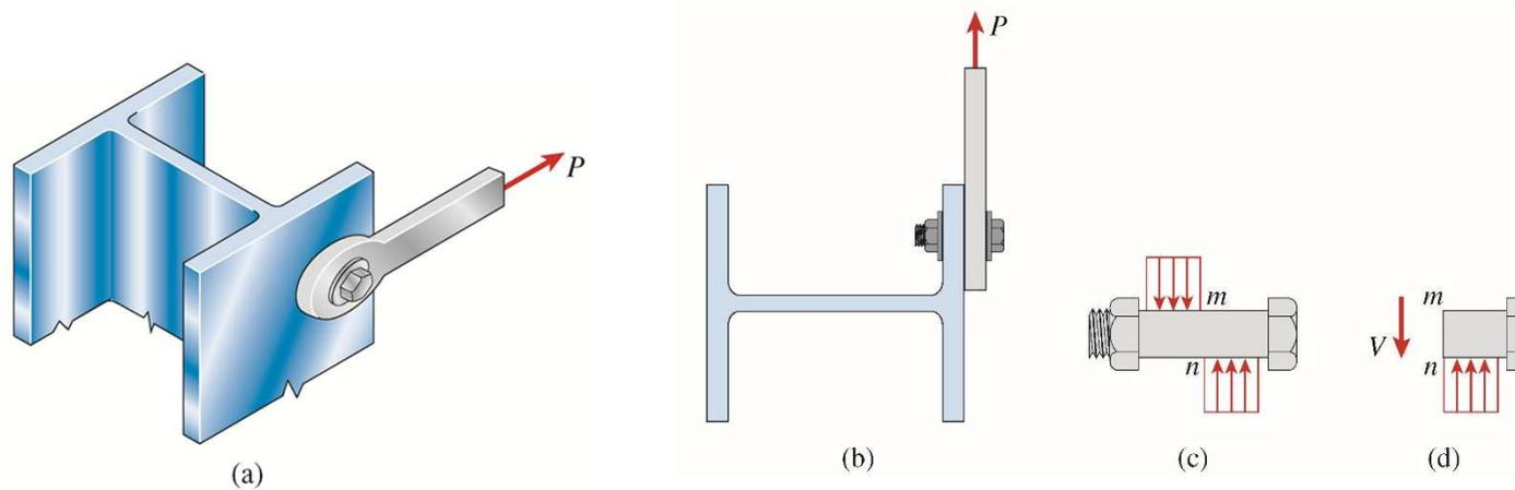
**FIG. 1-25** Bolted connection in which the bolt is loaded in single shear
