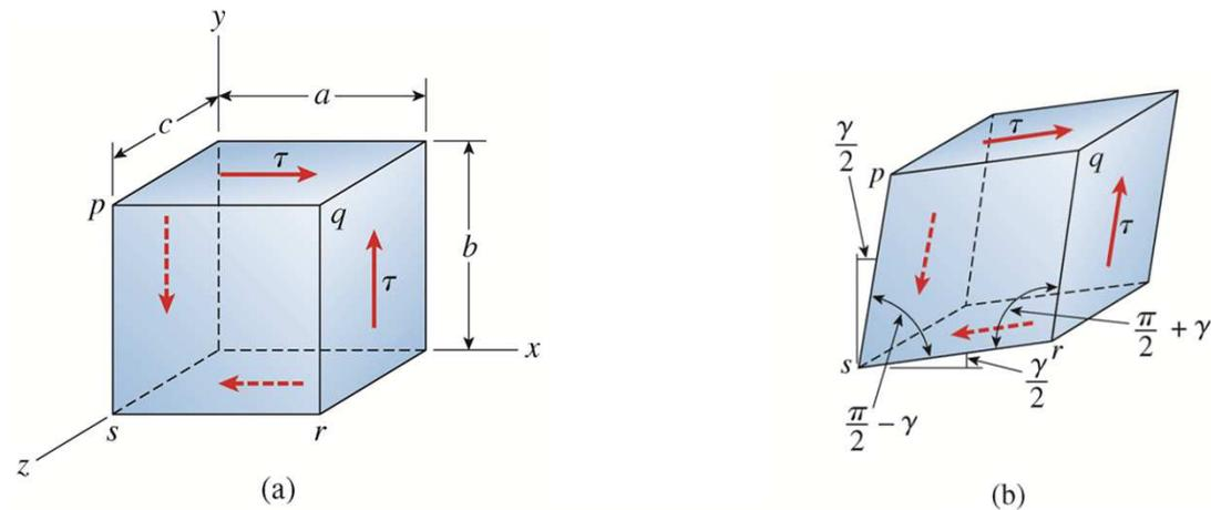
**FIG. 1-28** Element of material subjected to shear stresses and strains
