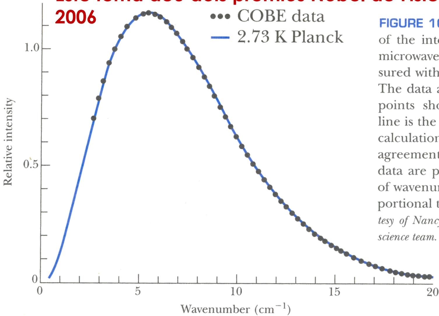
**FIGURE 16.15** The spectrum of the intensity of the cosmic microwave background as measured with the COBE satellite. The data are smaller than the points shown, and the solid line is the blackbody radiation calculation for 2.73 K. The agreement is spectacular. The data are plotted as a function of wavenumber (inversely proportional to wavelength). *Courtesy of Nancy Burgess, NASA COBE science team.*
