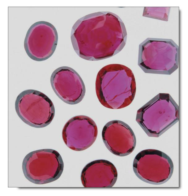
What makes a ruby red? The addition of about 1% chromium oxide in alumina creates defects. An electronic transition between defect levels produces the red ruby crystal. Similarly, incorporation of Fe<sup>+2</sup> and Ti<sup>+4</sup> makes the blue sapphire. (Courtesy of Lawrence Lawry/ PhotoDisc/ Getty Images.)
