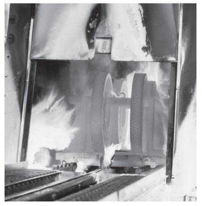
**Figure 5-1** Furnace for heat treating steel using the carburization process. (*Courtesy of Cincinnati Steel Treating.*)
