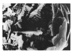
**Figure 9-26** Dendrites in a titanium powder particle produced by rapid solidification processing (× 2200) (for Problem 9-43). (*From J.D. Ayers and K. Moore, "Formation of Metal Carbide Powder by Spark Machining of Reactive Metals,"* in Metallurgical Transactions, *Vol. 15A, June 1984, p. 1120.*)
