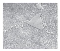
**Figure 14-7** (a) (Repeated for Problem 14-21.) Microstructure of a superalloy with carbides at the grain boundaries and  $\gamma'$  precipitates in the matrix (× 15,000). (*From* ASM Handbook, *Vol. 9, Metallography and Microstructure* (1985), ASM *International, Materials Park, OH* 44073–0002.)
