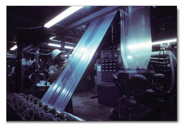
Polymers can be processed into a variety shapes through numerous manufacturing techniques. This photo shows the extrusion of a molten thermoplastic tube. Before the polymer fully solidifies, hot air is blown through the tube, as it moves vertically upward, causing it to expand up to several times in diameter. The flattened tube is then sealed on one side with heat and cut on the other to form plastic bags or simply cut along the length to form plastic sheet (©Bob Masini/Phototake).
