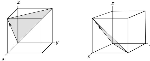
4-24 What are the Miller indices of the {110} slip planes in BCC unit cells that include the [111] slip direction?
