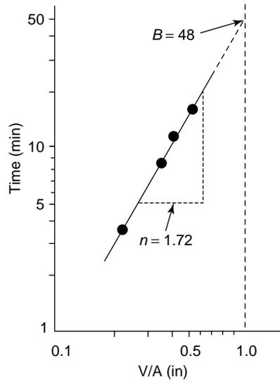
**8-34** Find the constants  $B$  and  $n$  in Chvorinov's rule by plotting the following data on a log-log plot.
