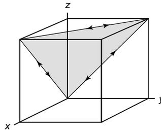
**3-64** What are the indices of the four directions of the form  $\langle 111 \rangle$  that lie in the  $(\bar{1}01)$  plane of a cubic cell?
