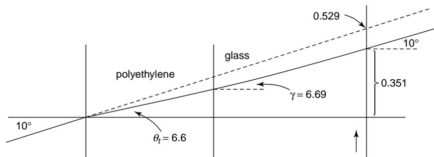
(a) As the beam passes from air into polyethylene (which has an index of refraction of 1.52),
