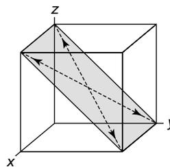
4-23 What are the Miller indices of the slip planes in FCC unit cells that include the [101] slip direction?
