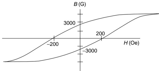
**19–28** A magnetic material has a coercive field of 10.74 A/m, a saturation magnetization of 2.158 Tesla, and a remanance induction of 1.183 tesla. Sketch the hysteresis loop for the material.
