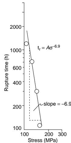
**6-106** Using the data in Figure 6-59(a) for an iron-chromium-nickel alloy, determine the activation energy  $Q_r$  and the constant “ $m$ ” for rupture in the temperature range 980 to 1090°C.
