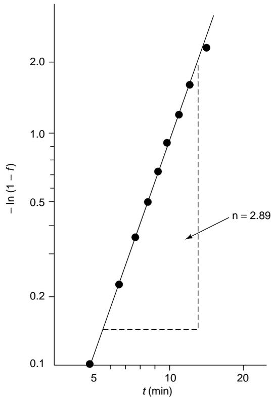
**11-3** Determine the constants  $c$  and  $n$  in Equation 11-2 that describe the rate of recrystallization of copper at  $135^{\circ}\text{C}$ . (See Figure 11-2)
