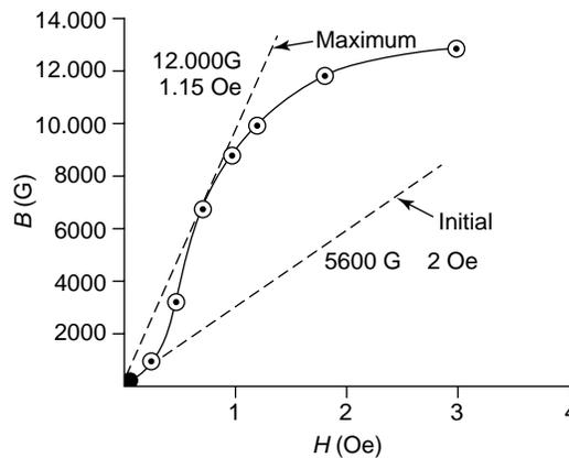
The data is plotted; from the graph, the initial and maximum permeability are calculated, as indicated:
