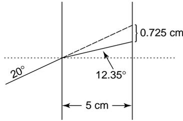
From the sketch, we can find the displacement of the beam expected if no refraction occurs:
