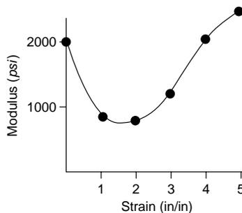
The modulus of elasticity is plotted versus strain in the sketch. Initially the modulus decreases as some of the chains become untwisted. However eventually the modulus increases again as the chains become straight and higher stresses are required to stretch the bonds within the chains.
