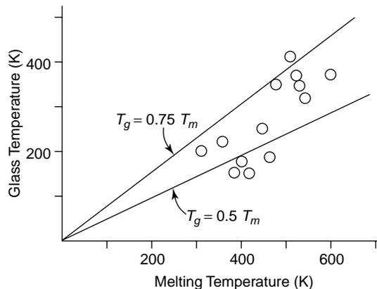
Most of the polymers fall between the lines constructed with the relationships  $T_g = 0.5T_m$  and  $T_g = 0.75T_m$ . The condensation thermoplastics and elastomers also follow this relationship.
