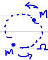
$$\text{Radiated Power} \sim \frac{G M^2 \Omega^2 (\Omega L)^4}{c^5}$$
