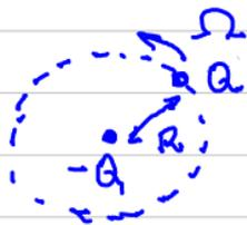
$$\text{Radiated Power} \sim \frac{k}{c^3} Q^2 \Omega^2 (\Omega L)^2$$
