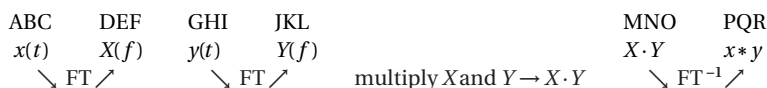
Fig. 7.5-1: The layout of the data in convolution exercise 7.5-1. The top row identifies the columns used, the middle row the functions encountered there, and the bottom row the mathematical operations between them. The data for X \cdot Y are computed as the products of the complex numbers in X(f) and Y(f) .
