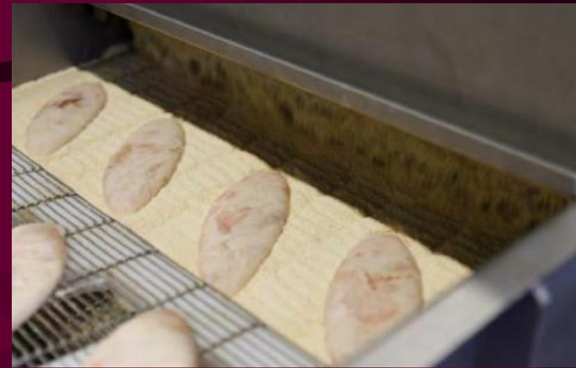
*Figure 10.4. Pre-Dust Application Using a Flatbed with an "Air Knife" Blowing Mechanism. Courtesy of Stein DSI, Sandusky, OH, U.S.A.*
