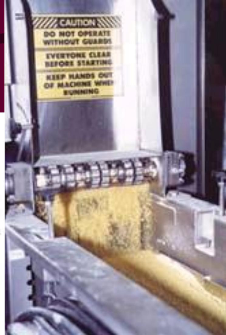
Figure 14.6.2.1 An example of a breading applicator for cracker type and home-style crumbs.
