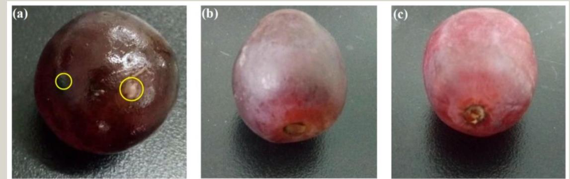
Preservation of red grape packed in different materials at 37°C for six days: (a) plastic wrap; (b) pure chitosan film; (c) chitosan-TiO<sub>2</sub> film.
