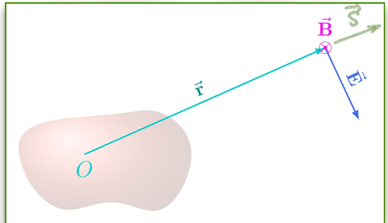
$$\frac{d^2 \vec{p}}{dt^2} \parallel \hat{z} \quad \Rightarrow \quad \begin{cases} \vec{E} &= \frac{\mu_0}{4\pi r} \left| \frac{d^2 \vec{p}}{dt^2} \right| \sin \theta \hat{\theta} \\ \vec{B} &= \frac{\mu_0}{4\pi r c} \left| \frac{d^2 \vec{p}}{dt^2} \right| \sin \theta \hat{\phi} \end{cases}$$
