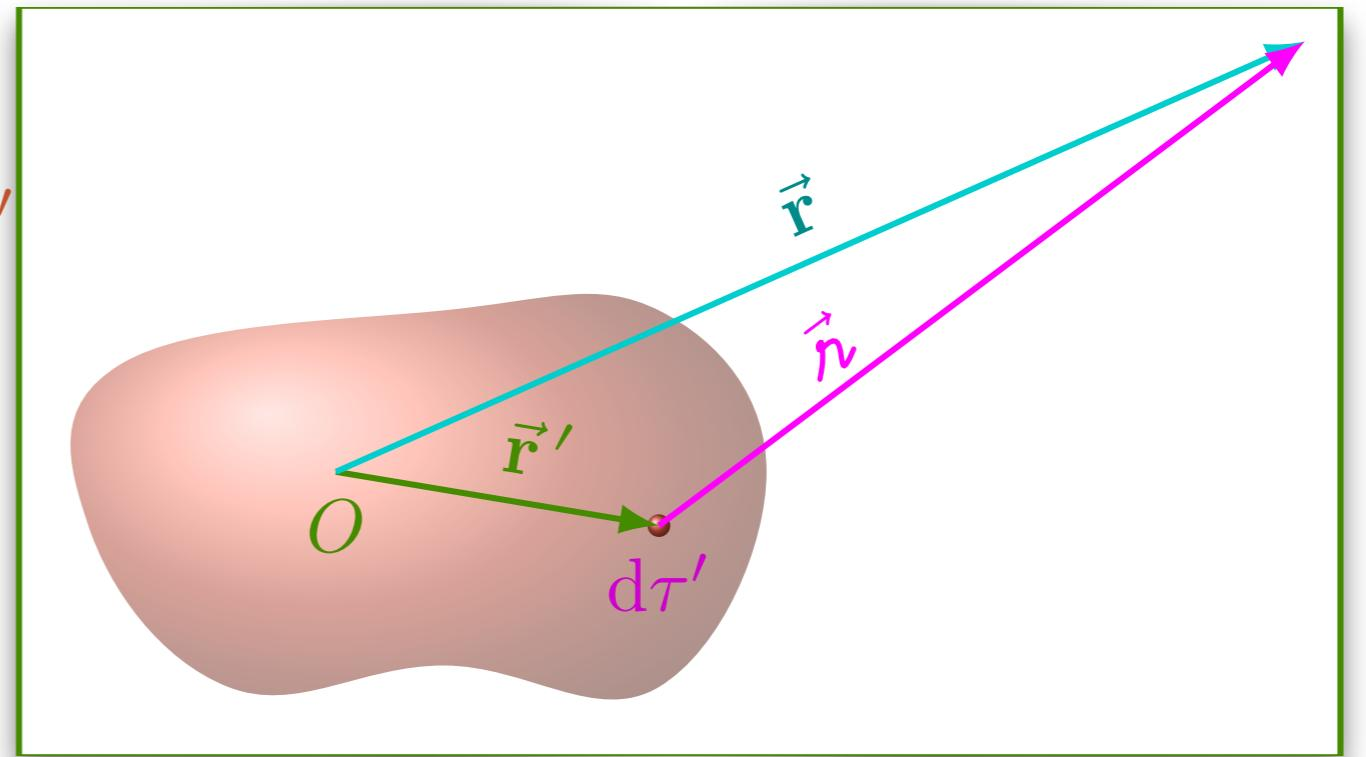
$$V(\vec{r}, t) = \frac{1}{4\pi\epsilon_0} \left( \underbrace{\frac{1}{r} \int \rho(\vec{r}', t_0) d\tau'}_{Q \text{ (CARGA)}} + \underbrace{\frac{\hat{\vec{r}}}{rc} \cdot \frac{d}{dt} \int \vec{r}' \rho(\vec{r}', t = t_0) d\tau'}_{\vec{P} \text{ (MOMÉNTO DE DIPOLO)}} \right)$$
