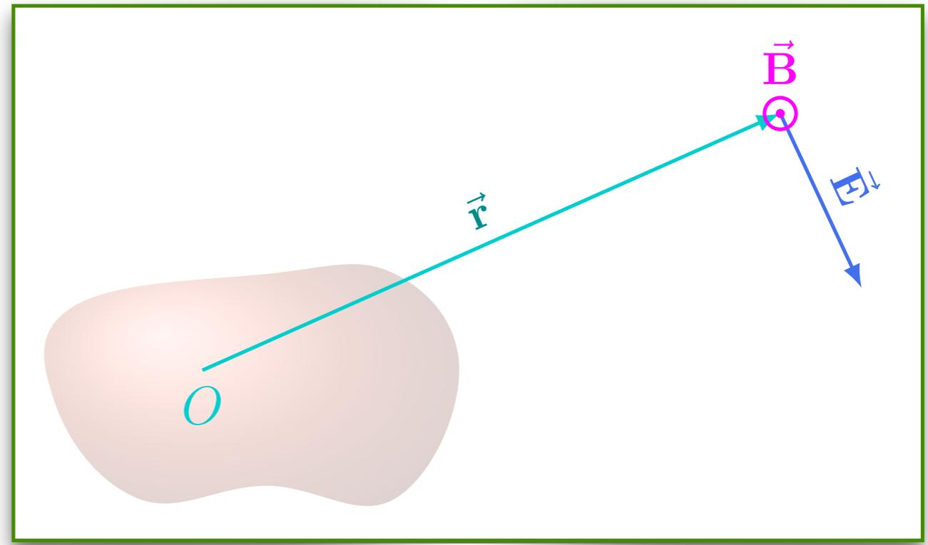
$$\frac{d^2 \vec{p}}{dt^2} \parallel \hat{z} \Rightarrow \left\{ \begin{array}{l} \vec{E} = \frac{\mu_0}{4\pi r} \left| \frac{d^2 \vec{p}}{dt^2} \right| \sin \theta \hat{\theta} \\ \vec{B} = \frac{\mu_0}{4\pi r c} \left| \frac{d^2 \vec{p}}{dt^2} \right| \sin \theta \hat{\phi} \end{array} \right\}$$
