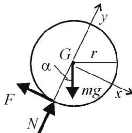
$$\text{TR: } m\vec{a}_G = (mg \sin \alpha - F) \vec{I} + (N - mg \cos \alpha) \vec{J} \quad (\text{A})$$
