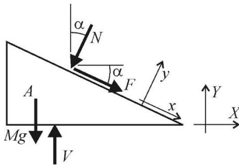
$$\begin{aligned} \text{TR: } M\vec{a}_A &= M a_A \vec{I} = (F \cos \alpha - N \sin \alpha) \vec{I} + \\ &\quad + (V - Mg - N \cos \alpha - F \sin \alpha) \vec{J} \Rightarrow \\ &\Rightarrow M a_A = F \cos \alpha - N \sin \alpha \end{aligned} \quad (1)$$
