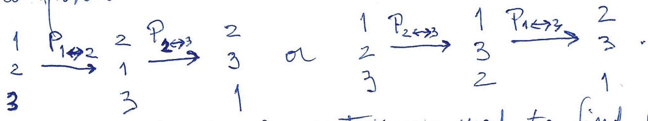
This is the kind of matrix we need to find in PA=LU. In the general case is composed of several elementary permutation matrices  $P_k$ . Such matrices perform only one row/col switch each time.
