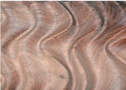
CNC machining is increasingly accessible in schools as well as industry. The CNC is programmed first to do a roughing operation with a larger cutter to remove as much material as possible. This is followed by finer mill cutters that remove smaller but more exact amounts of materials before the final sanding coat. See Chapter 8 on CNC machining and laser cutting (page 74).
