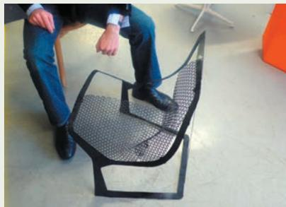
An early prototype for the Myto chair made from cardboard and perforated sheet metal was used to explore the overall form factor and design strategy. This model was reverse-designed into CAD using measurements.
