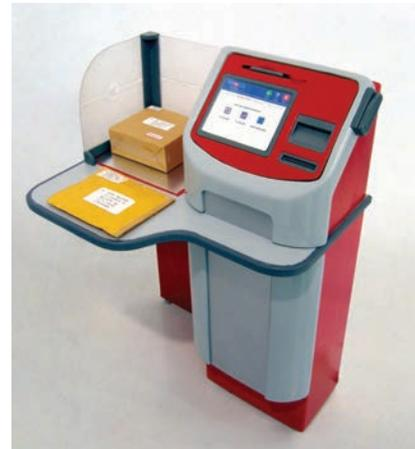
Full-scale prototypes help to finalize task flow and design requirements. The fidelity is gradually increased as more details are resolved.
