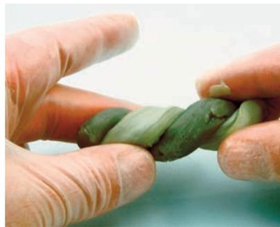
Part A and Part B are kneaded together by braiding and folding until color is consistent.
