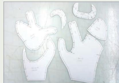
The paper prototype is cut apart along the seam lines. These pieces were traced on new paper, adding seam allowances and notches. This was the first set of patterns (above right) and was now ready to be transferred to neoprene.
