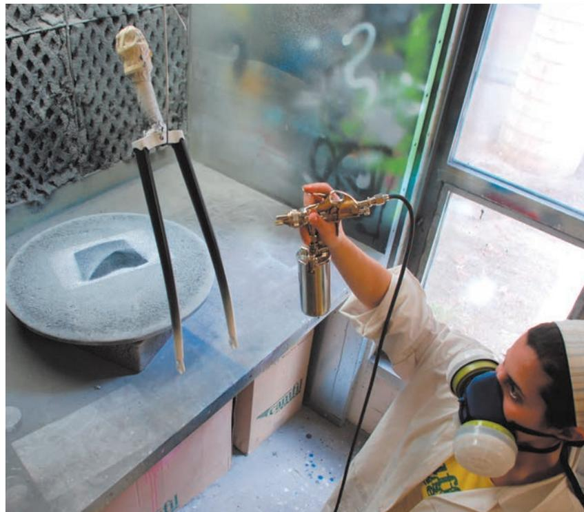
compressor has an air-pressure tank that regulates the air pressure, as well as a pressure valve and a moisture trap to capture water droplets before they enter the airstream. The compressor will be adjusted somewhere between 20 and 40PSI. A flexible hose is then connected to the sprayer.
