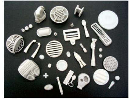
Such parts as these can be printed in a matter of hours, allowing students to incorporate more detail into their projects.
