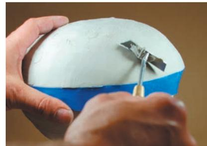
**Step 5** The top surface is finally slicked with a 0.008in (0.2mm) thick spring-steel slick. It is important to work in different directions with the slick in order not to establish a low spot.
