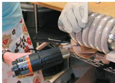
A barbecue utensil is heat-formed with a strip heater and handheld heat gun. Plastic tubes can be thermoformed without collapsing by first filling them with sand and capping the ends (left).
