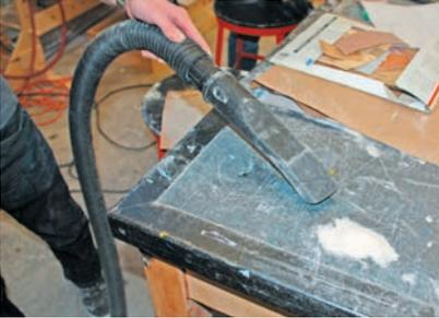
Dust may also be generated when working by hand. This is especially true when using modeling-foam materials, which cling to everything. It is important to keep the dust from accumulating by regularly vacuuming the area.
