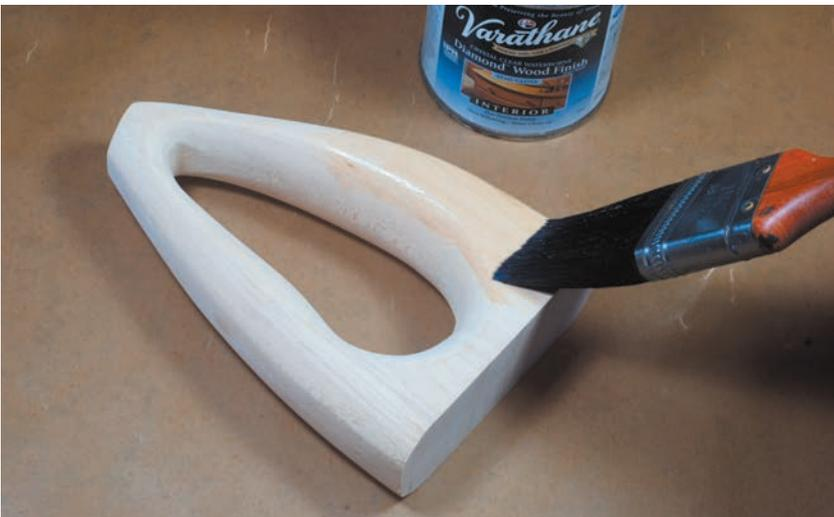
Sealing wood with several layers of water-based polyurethane ensures that the wood grain is hidden when painting.
