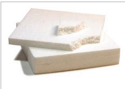
Expanded polystyrene foam is less suitable as a modeling material owing to its beaded construction.
