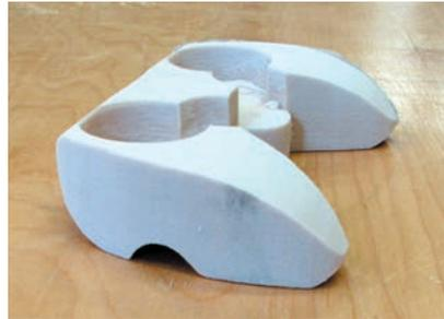
**Step 9** The finger-rest concave surface is sanded with a post sander. This could also be done with a circular-shaped rasp.
