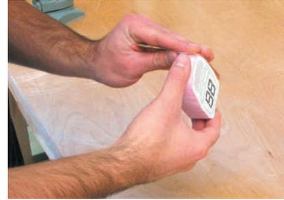
**Main Body Step 3** In order to create the convex top surface, the transition is marked with masking tape. A top label is also added that defines the top LCD plane.
