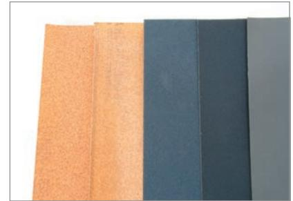
Different grit sandpapers are required for modelmaking. A basic toolset includes a range of coarse to fine sandpaper.
