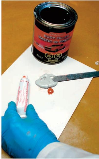
Automotive body filler is mixed according to the manufacturer's instructions. It is important to achieve a uniform color consistency to ensure that mixing has been thorough.
