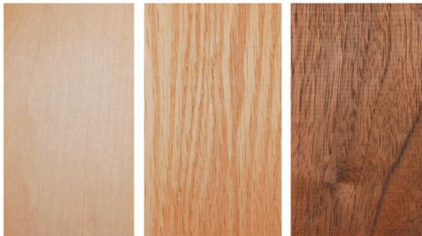
Wood is graded for different applications and markets. Construction lumber is likely to be fast-growing softwoods, such as spruce, and is likely to have knots and splits. Furniture-grade wood is selected not to have deficiencies and is also kiln-dried, making it resistant to splitting and shrinking. There is an associated trade-off in cost and availability.
