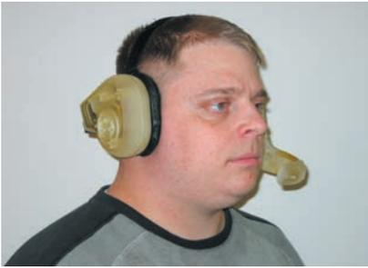
The comfort of each of the redesigned Motorola headsets for the NFL was verified through prototyping.
