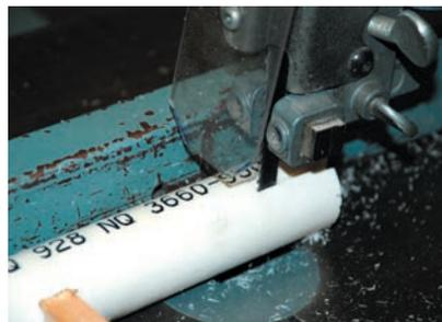
**Rubber Handles Step 1** The rubber handle pieces are simulated using a plastic tube. The cross sections of the handle pieces correspond to a section of a cylinder. 1.5in (3.8cm) diameter plastic tubing is trimmed on the bandsaw. It is essential to have adequate training and supervision when using power equipment such as a bandsaw. Note how the lateral push stick has a V-notch taken out of it to hold the circular tube better.
