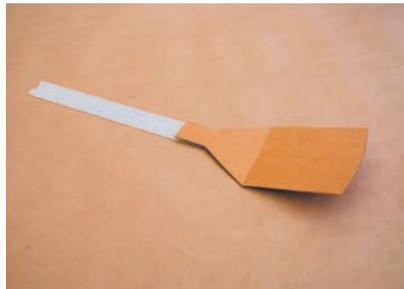
**Spatula Step 1** The spatula shape is cut out from acrylic sheet on a laser cutter. Two variations of the design are initially cut out to examine visual alternatives. The file for the laser cutter is an Illustrator® drawing.
