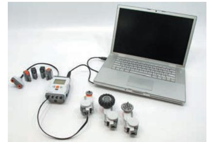
Lego Mindstorms® NXT is a stand-alone controller with an easily programmable interface. A variety of sensors, including touch, infrared, range, and sound, can be used to produce output including servomotors. It is programmed through a computer.
