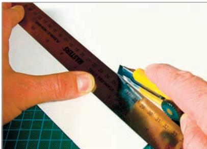
Utility and X-Acto knives are essential paper-modeling tools and should be kept sharp with an ample supply of replacement blades. Use a metal ruler and keep fingers away from the path of the cut.
