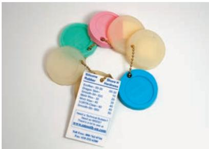
Rubber can be cast in a wide variety of stiffnesses, colors, and levels of transparency, as shown in these Silicone samples from Smooth-On, Inc.
