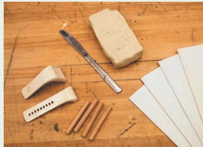
Materials are gathered for moldmaking. The wristband pattern is a rapid prototype that has been finished to a high level of fidelity through sanding, filling, and painting.
