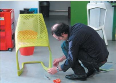
A final prototype of the Myto chair was made using the laser-sintering process. This prototype receives some final tweaks before the production tooling is made.
