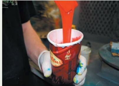
The mold is now ready for casting silicone wristbands. Clear silicone is mixed with custom colorants.
