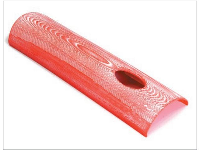
**Step 1** The part is first filled with spackle and then sanded smooth (see Chapter 9, page 83). If the part does not feel smooth to the touch, repeat the process.
