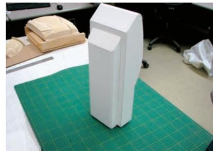
**Final Assembly Step 2** The final step is to glue on the decal that captures the interactive elements of the self-serve kiosk. Spray glue works well, but should be used only in a spray booth or outdoors. Double-sided tape or rubber cement are suitable substitutes.
