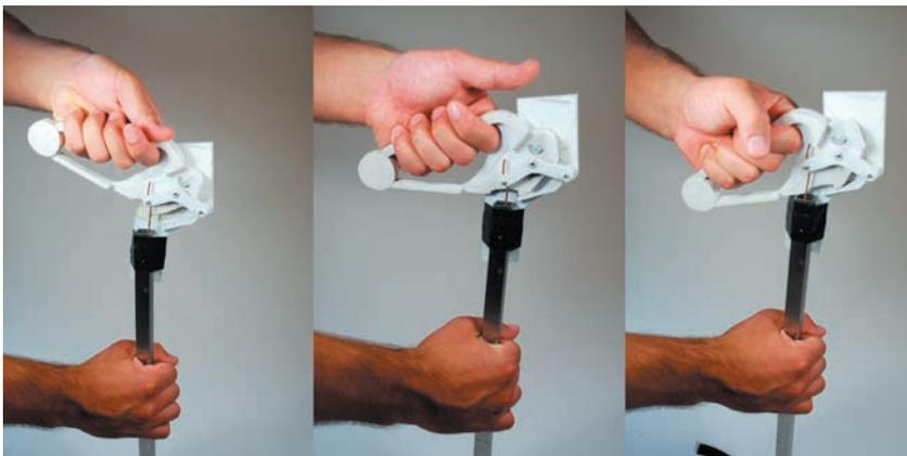
A proof-of-concept model brake mechanism made from styrene sheet. This handmade works-like prototype could be altered quickly to better understand the design parameters for a new internal brake mechanism for a rollator (rolling walker).
