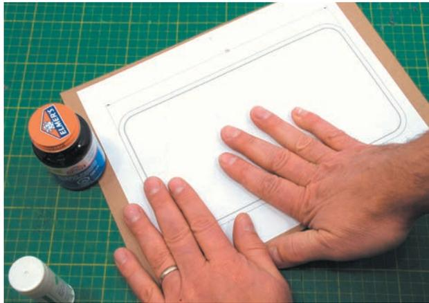
**Step 2** In order to add some stiffness to the model, the bottom is glued to a piece of cardboard.
