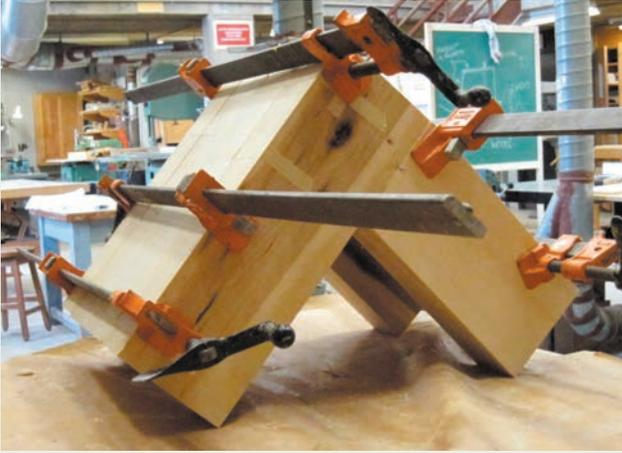
The vacuum-forming mold was made by laminating pieces of wood and shaping with rasps, sanders, and templates.
