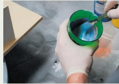
The first half of the mold is now poured, starting in a corner so as not to trap air bubbles.
