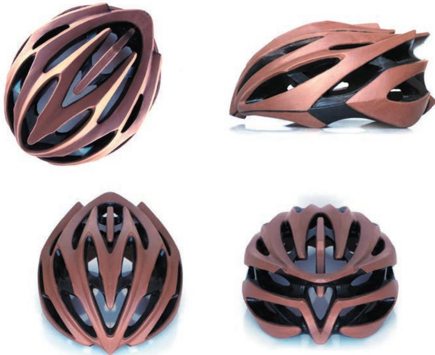
Clay is often the material of choice to develop highly complex organic forms, such as this helmet by Alan Okamura for the Spanish bicycle-gear company Spiuk. The helmet clay model was made using styling clay, which can also be painted.
