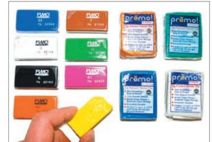
Polymer clay is available in various colors and hardens when baked. Small, detailed parts, such as this series of children's stationery items (tape dispenser, stapler), can be easily modeled by hand in polymer clay.
