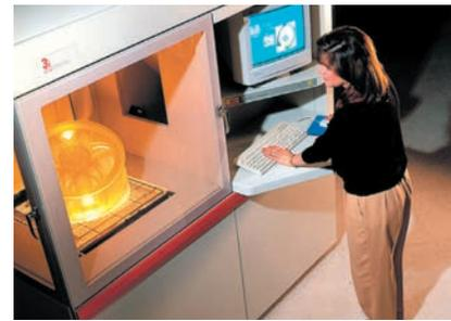
Stereolithography machines from 3D Systems, such as this SLA7000, produce parts from laser-cured photopolymers.
