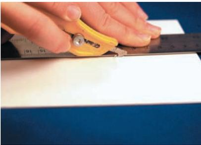
Thin styrene sheet is easily scored and then snapped (left), or cut with an X-Acto blade (right) for curved outlines.
