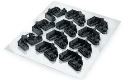
Small-scale production of parts in real plastics saves money on injection-mold tooling.
