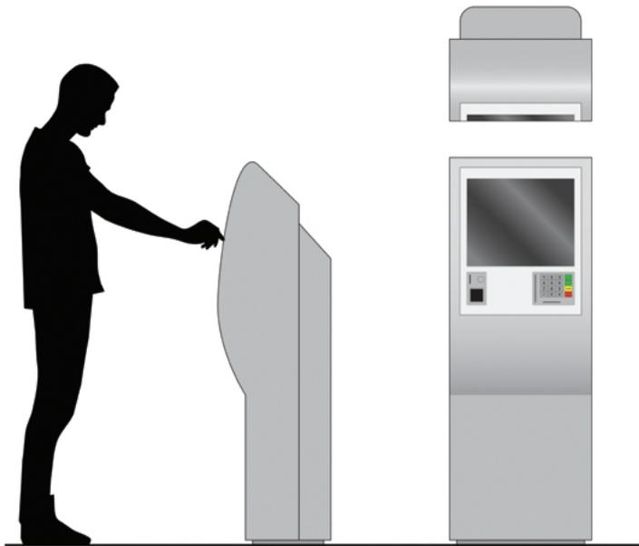
**Step 2** This exploded sketch shows that the kiosk model consists of two sections: a curved front interactive panel and a rear housing section. In terms of manufacturing we are simulating a product that would be made out of plastic and sheet metal.
