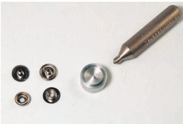
Snaps need to be riveted in place and consist of four parts.
