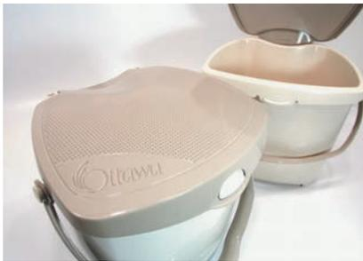
DW Product Development used casting to produce small numbers of the SureClose compost bin. This was helpful in verifying many design aspects before injection-mold tooling. The high-quality castings are visually and functionally equivalent to production parts, capturing fine details such as the debossed city logo, as well as the fine mesh of ventilation openings. These parts were outsourced to a company specializing in casting.
