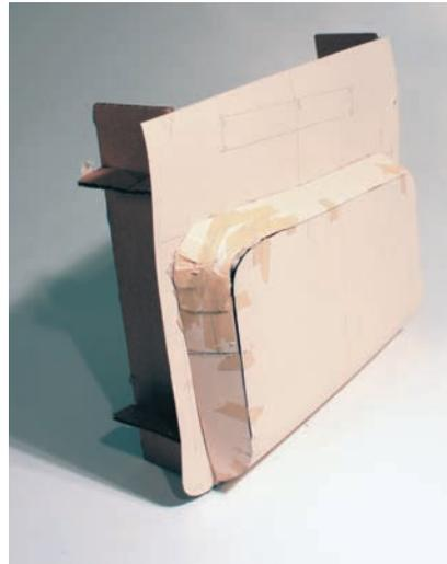
Cardboard is used to establish fit and dimensions for a laptop bag. Details on paper models are penciled in.
