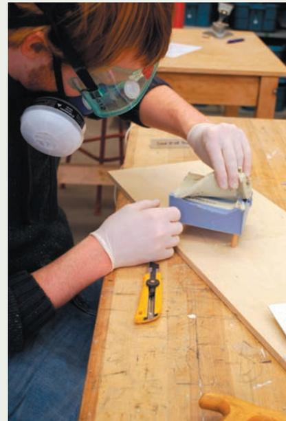
The process is now repeated in reverse. Note that small plasticine shapes have been added to the patterns in order to create the sprue and vent on each part.
