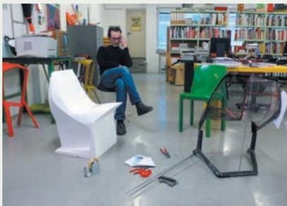
A solid Styrofoam model (shown in white) was used to verify the shape of the seating surface.
