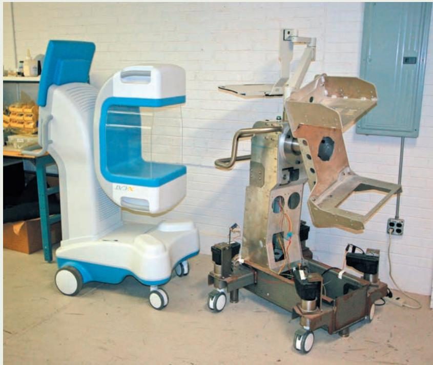
Looks-like versus works-like prototype of the frame.
