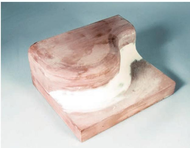
**Step F** The final shape should feel smooth and is then ready for priming. Half the model has been painted to show what the form will look like. A few coats of primer confirms whether more filling is necessary.
