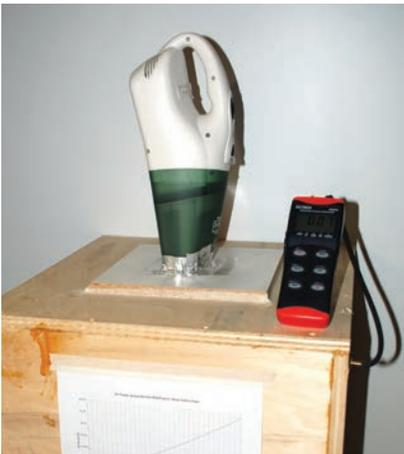
This test setup was built by FilterStream to test the suction of its handheld vacuums. The amount of suction inside the box is measured while the vacuum is running to verify performance.
