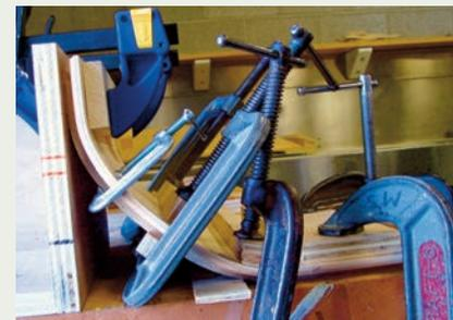
Clamps hold two pieces of wiggle board together during the lamination process.
