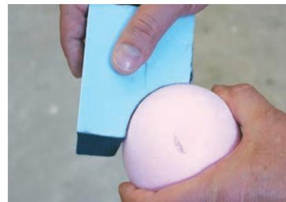
A polystyrene sphere is made by rasping the overall shape, followed by successively finer grades of sandpaper and a sanding template.
