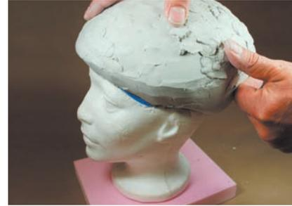
**Step 3** The helmet shape is initially carved with a toothed rake that removes effective amounts of clay. Typically, this also reveals low spots that have to be filled with more clay. It is advisable first to heat the model slightly in order to improve adhesion of the new layer of clay.
