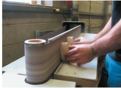
**Step 8** The side profile is then sanded to shape on a belt sander. This could have been done with a handheld rasp instead, in which case the part would be mounted in a vise while being worked on.
