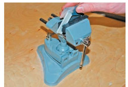
A sturdy bench vise provides secure holding of the workpiece (top), while a universal vise is useful for finer, more delicate work (above).
