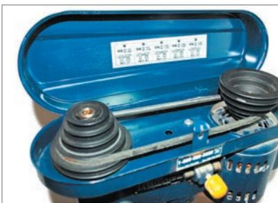
Drill press speed can be adjusted through a pulley arrangement between the motor and spindle. This should only be done when the machine is stopped and unplugged. The chart on the bottom of the guard cover on this machine shows speed options.
