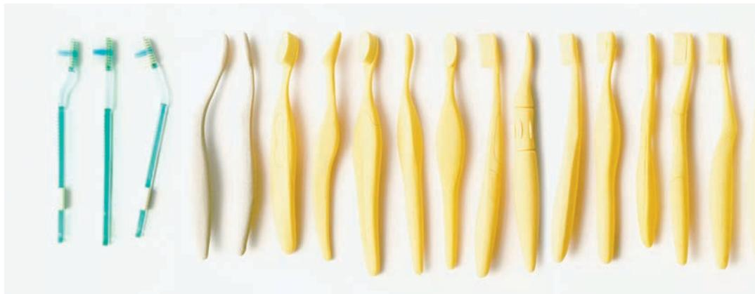
obvious how the early prototypes looked at options for the overall shape, whereas the later models made in harder, more exact materials included coloring and textural detailing. This is precisely why prototyping is both iterative and progresses from low to high fidelity.
