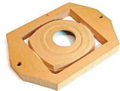
A thin-walled part machined on a three-axis machine. The top is machined and then the part is flipped over to machine the bottom. Note the two holes that are used for registration and the small amount of material that allows the part to hang on the frame.
