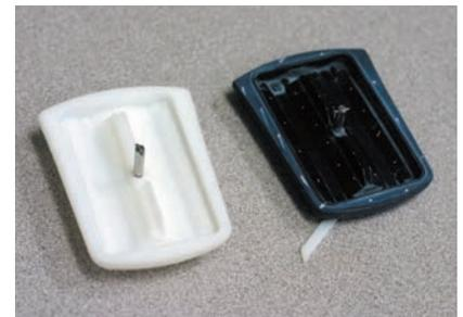
The new battery door (white) was printed on a Dimension 3D printer, based on data scanned in from the original battery door (black).
