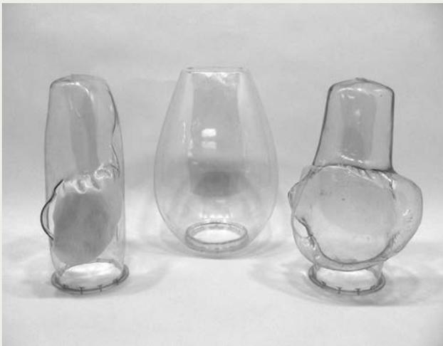
Sometimes a design presents manufacturing challenges. In these cases, it is important to verify that the shape can be made. Establishing that the Luau™ lantern body could be blow-molded required some manufacturing experimentation.
