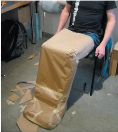
A prototype for a rain-protection garment for wheelchair users is tried out first in paper.
