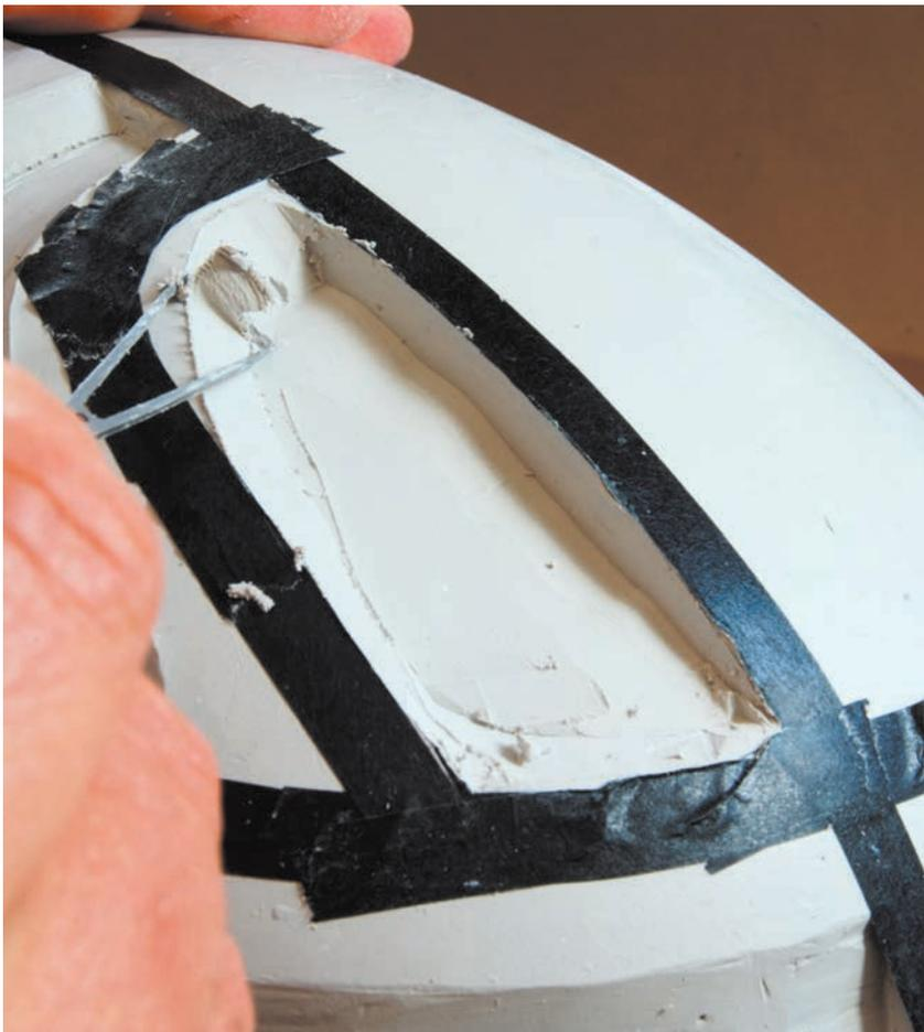
**Step 9** The final ventilation surfaces are added in the same manner, using tape to define edges and protect existing surfaces. Note how only half the helmet is detailed in order to avoid issues of symmetry and to save time.
