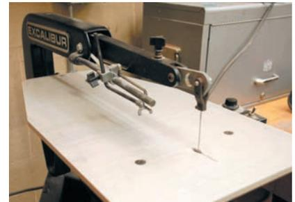
The scroll saw produces intricate contoured cuts
