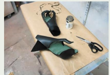
A sewn neoprene prototype is shown left. The seam lines are glued with a rubber sealant and trimmed short to replicate a bonded seam construction.
