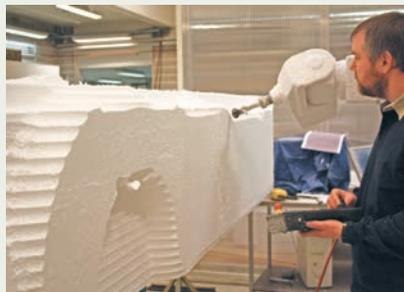
A large five-axis Kolb CNC machine was used to mill a full-scale model out of a large block of polystyrene foam.
