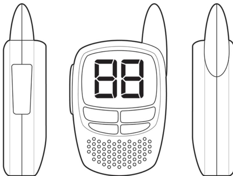
**Main Body Step 1** The top view of the model is glued to the foam with glue stick or rubber cement (these types of glue allow the label to be peeled off later). Next the profile is cut using a hotwire, leaving a little extra material for finishing. Be sure to do some testing with feed and voltage on a scrap piece beforehand. The outline could also be cut on a bandsaw, scroll saw, or even by hand.
