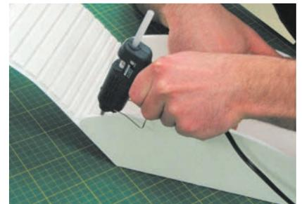
**Rear Housing Step 1** The sides and back are created in one piece of foamcore. The rear corners are rounded, which requires three V-notches to be removed on both corners.
