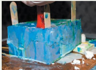
The silicone is injected into the mold with a syringe. The mold is filled through the sprue until the mold is full and material exits at the vent.
