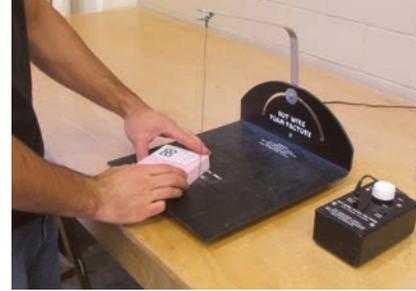
**Main Body Step 2** The hotwire trims the part to size, but leaves a coarse outline. The extra millimeter of material should be left so that it can be smoothed with 320-grit sandpaper. The top outline template will be peeled off for the next step.
