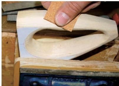
Once the shape has been roughed in, it is time to move to sandpaper, starting with a coarse 80-grit paper and progressing toward finer grades (120, 240 grit).
