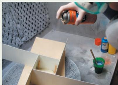
A spray-on mold release is applied. This helps in the removal of the pattern at the end.
