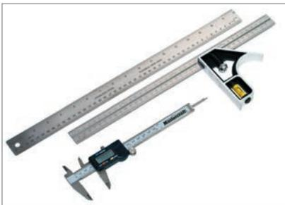
Steel rule (top), steel square with adjustable base (middle), electronic vernier caliper (bottom).
