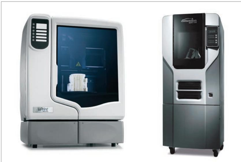
Dimension 3D printers use real ABS plastic to create parts.
