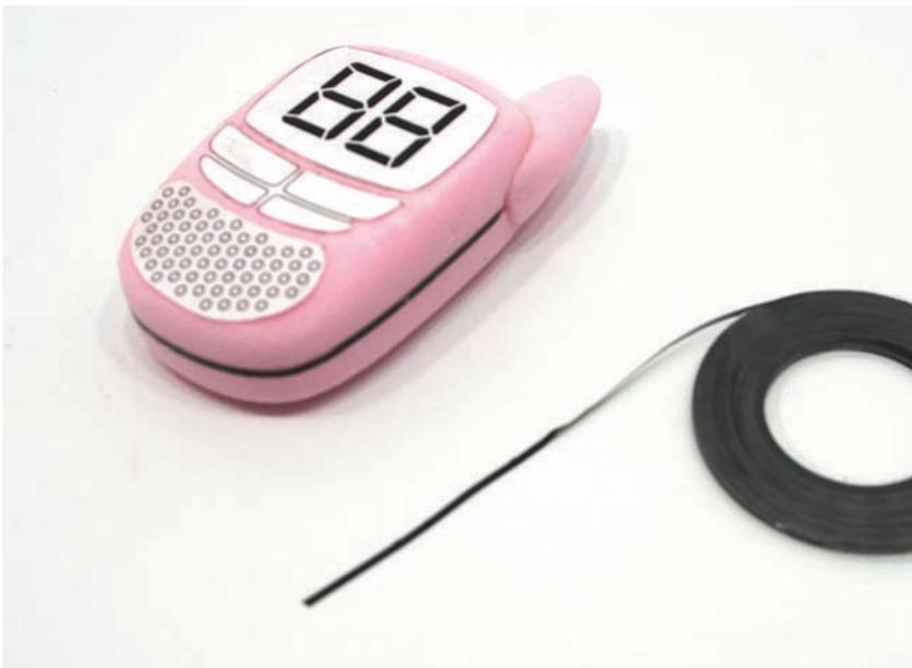
**Final Assembly Step 3** Thin graphic design tape is applied to define the parting line as shown.
