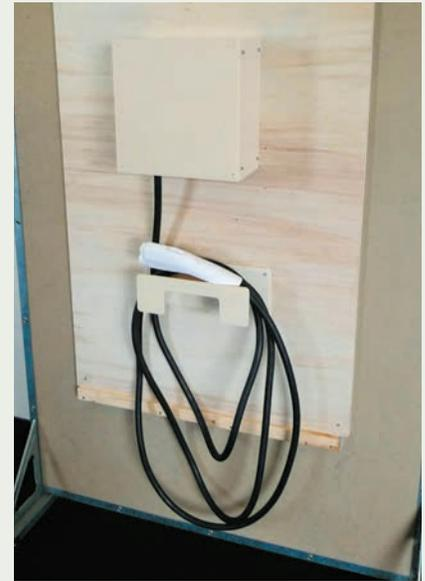
Low-fidelity full-scale prototypes were useful for user testing and showed that the residential cable wrap should be kept very close to the wall and separate from the charger housing.
