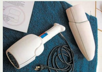
A more robust wooden prototype was used to test the new configuration with end users. At the same time polystyrene foam models were made to study form (above)
