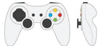
**Step 1** The process starts with sketching the form of the product. Scale top and side views will be used as cutting templates. These can be hand-drawn or created in Illustrator®.
