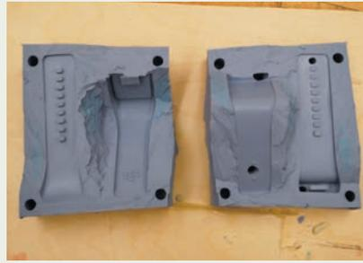
The mold is now complete. Note the sprue and vent openings on the part.
