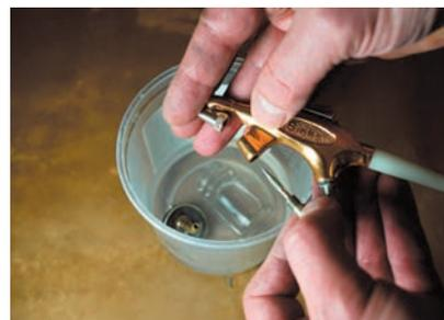
The airbrush should be cleaned after each paint application. Before the airbrush is put away, it is disassembled and thoroughly cleaned according to manufacturer's instructions.
