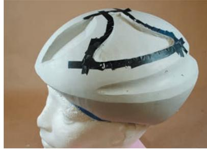
**Step 7** The top vent depression is a bit more complicated and requires a two-step process. First, rice-paper tape is used to define the edge of the surface depression. This depression is then carved out to the desired depth.
