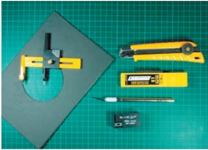
A utility knife and X-Acto cutter should be stocked with extra blades and used on a cutting mat.
