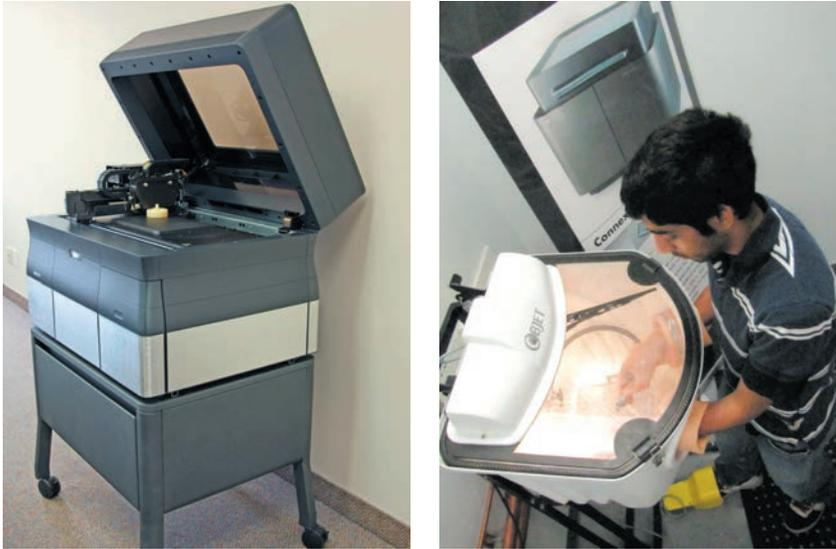
The Objet30 3D printer from Objet Geometries produces acrylic parts made from UV-cured photopolymers. The support system is cleaned off in a wash station (left).
