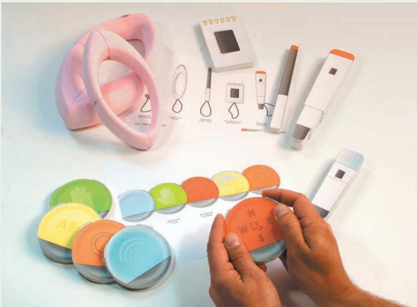
Exploratory prototypes were made in foamcore and Styrofoam to allow team members to develop interaction scenarios that could be studied further.
