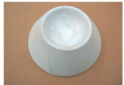
This bowl-shaped vacuum-forming mold was made on the wood-turning mill using a computer-generated template as a guide.
