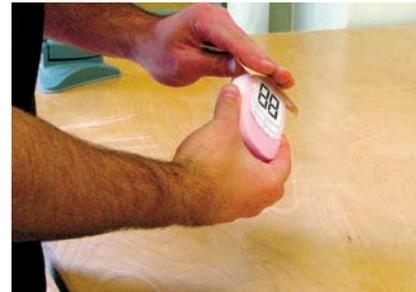
**Main Body Step 4** The convex top surface is carefully shaped with 320-grit sandpaper. Since the paper label resists sanding more than the foam, the transitions are kept crisp and clean.
