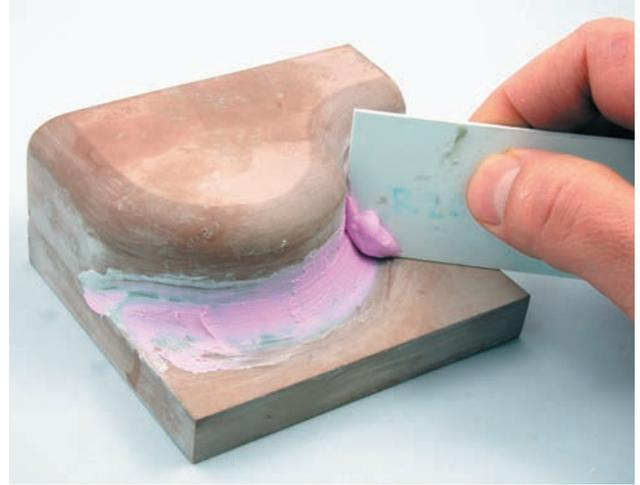
**Step D** Quick-drying spackle is used for final finishing. The DryDex® brand of spackle contains a colorant so that it starts pink and hardens to a white color.
