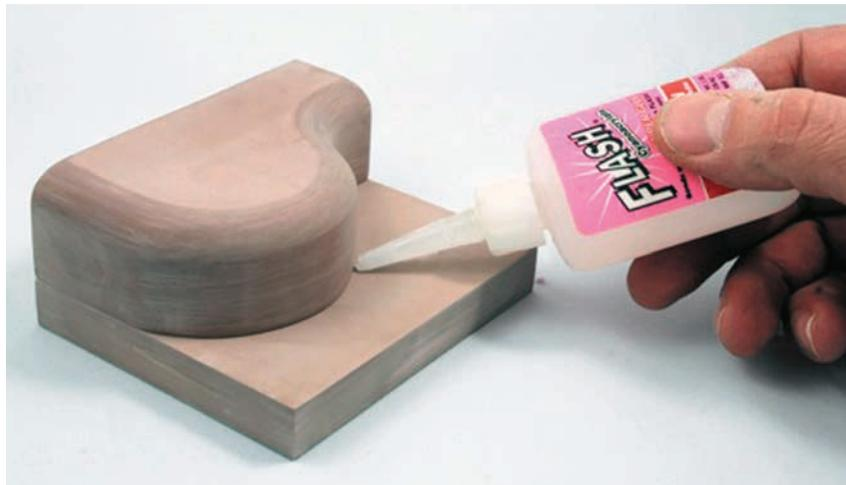
**Step A** The two parts are aligned and glued with a thin cyanoacrylate glue that wicks between the two parts.
