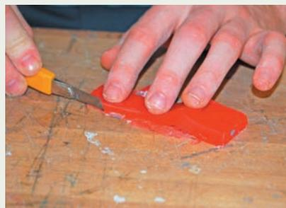
After the silicone sets, the mold is taken apart to free the parts. Flash at the parting line is trimmed off carefully afterward.
