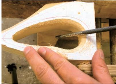
The rasp is a fast and effective tool for rough shaping. Pieces should be clamped securely. A round rasp will work better on inside corners, as shown on the handle opening below left.
