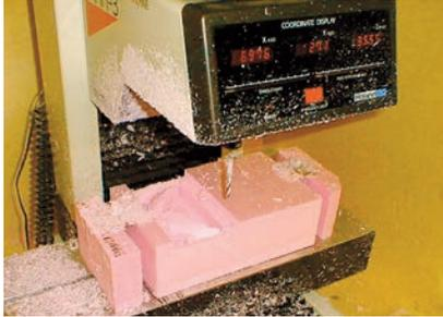
A part is quickly machined in Styrofoam to check the tool path.
