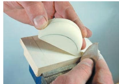
The three-step approach as shown here involves cutting with a saw, shaping with a rasp, and finishing with sandpaper.
