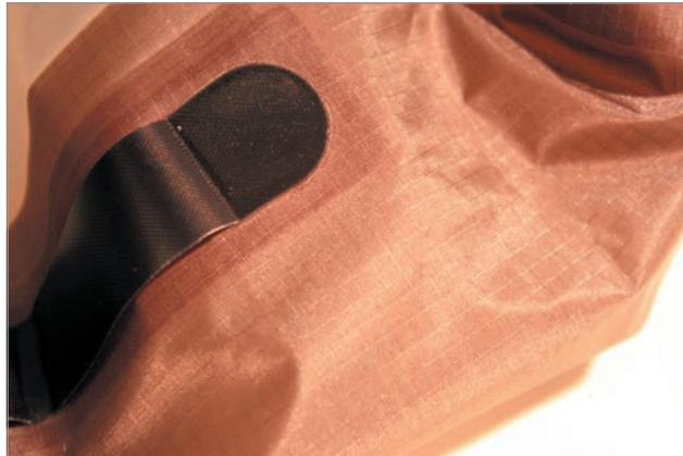
**Glued Seams** Certain seams are glued in order to replicate more advanced production techniques such as RF (radio frequency) welding or heat bonding. RF-welded seams are most common where a product must be completely airtight or watertight. One can imitate the effect by overlapping and gluing weldable fabrics together, such as neoprene.
