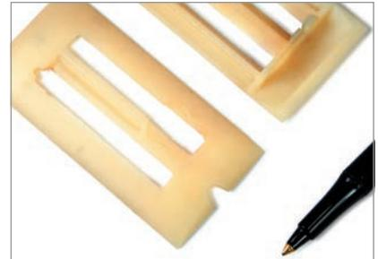
Fine-detail CNC-machined ABS prototype. These parts were machined with a very fine-ball end-mill cutter (0.06in/1.5mm dia.).
