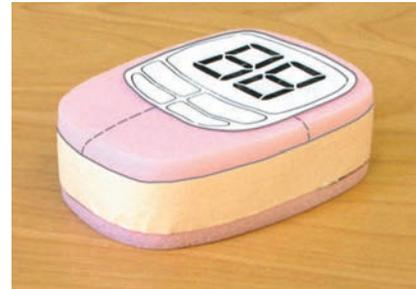
**Main Body Step 5** A side-profile template can be used to check that the profile is as intended. This step is not strictly needed, but helps maintain a predefined shape. A new top label will later need to be printed and applied, since the label has been sacrificed during sanding.
