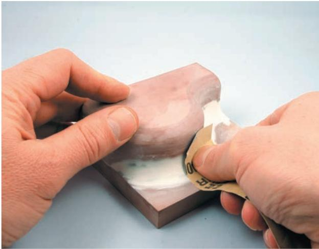
**Step E** Sanding with 400- and 600-grit sandpaper ensures complete smoothness. The final inside fillet radius is checked with a template. Filler application is repeated if necessary.
