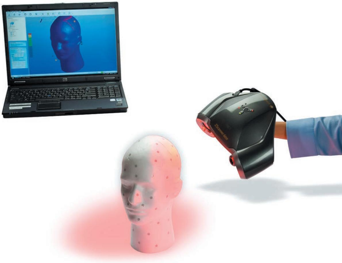
The handheld ZScanner® 600 from Z Corporation allows automated continuous scanning without post-processing.
