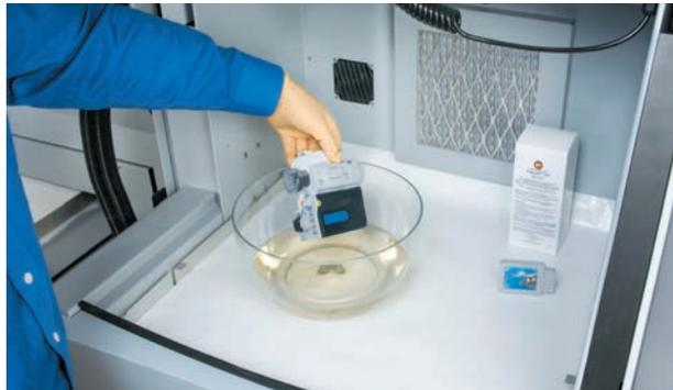
Parts are infused with salt water, cyanoacrylate, or two-part epoxy depending on the intended use and application.
