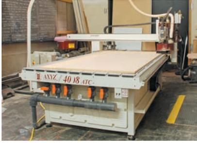
Wood routers are often used to cut outlines in sheet material, but some have a third axis to be able to control the vertical dimension.
