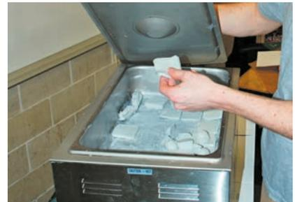
Clay billets are usually cut into smaller parts and softened in an electric chafing dish. Make sure to keep temperature at or below the manufacturer's suggested temperature.
