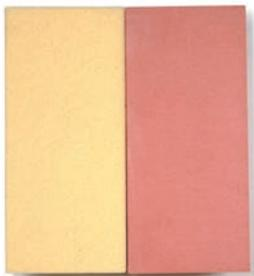
15lb/ft<sup>3</sup> (240kg/m<sup>3</sup>) PU foam (left) and 30lb/ft<sup>3</sup> (480kg/m<sup>3</sup>) machining board (right) are common low- and high-fidelity material choices respectively.
