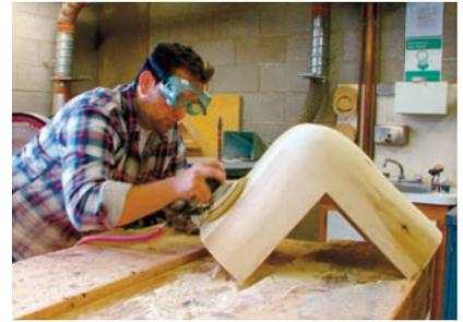
Preparing a vacuum-forming tool out of wood.
