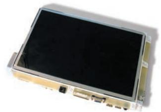
The accuracy and strength of this SLS prototype for the Motion Computing J3400 tablet allowed mechanical testing at the critical stage of design and engineering implementation.
