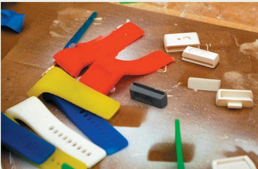
The same mold is used to cast a variety of wristbands in different colors.
