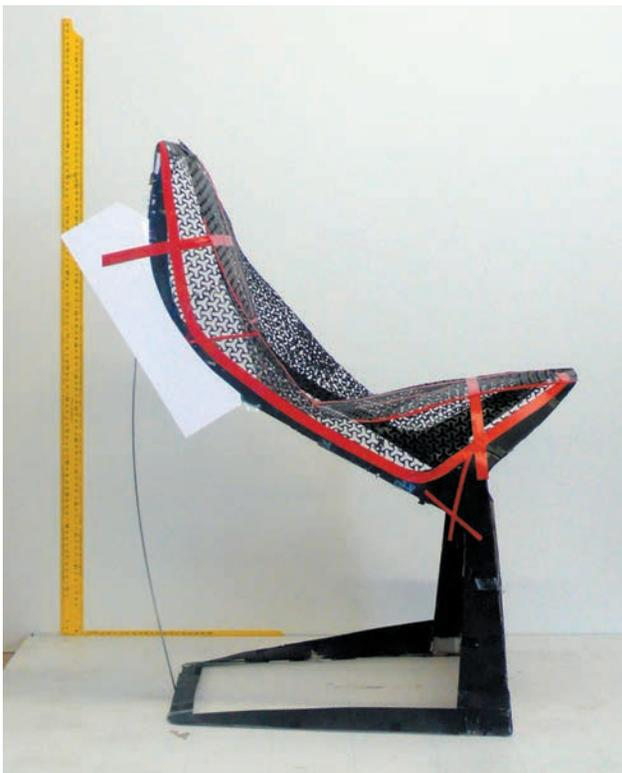
Konstantin Grcic reverse-designed the first Myto chair prototype as a starting point for CAD.
