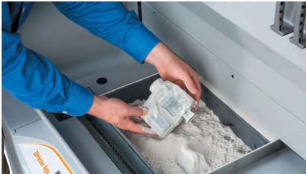
The printed part is removed from plaster build tray.
