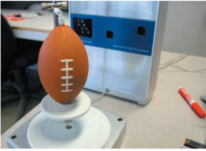
The NextEngine stationary desktop scanner includes a rotating mounting base that automatically rotates the object to be scanned.
