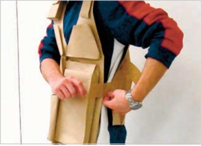
Paper prototypes often precede fabric prototypes when exploring new sewn products and are used in pattern creation.
