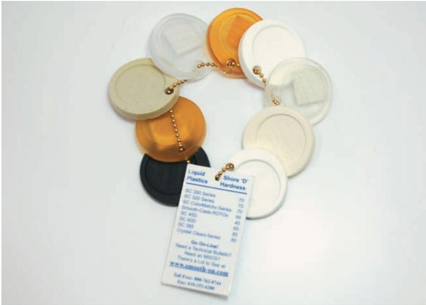
Polyurethane can be cast in a number of colors, and with a variety of structural properties and degrees of clarity as shown in these samples from Smooth-On, Inc.
