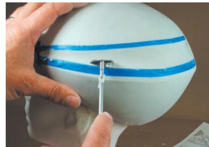
**Step 6** The concave side-ventilation opening is added. The ventilation features will be added only to one side of the helmet. Tape is used to define the edge, and various tools are used to remove material to the desired shape.
