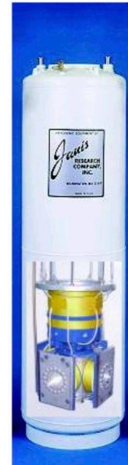
Superconducting magnet  $10 \text{ T}$
