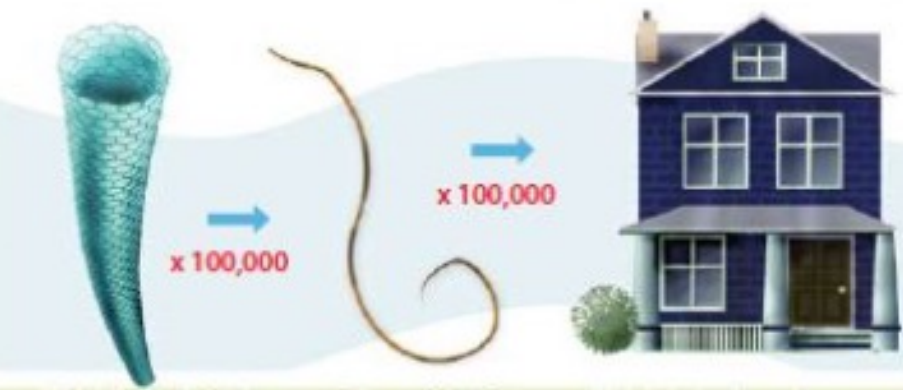
Single-walled Carbon Nanotube 1 nanometer diameter
