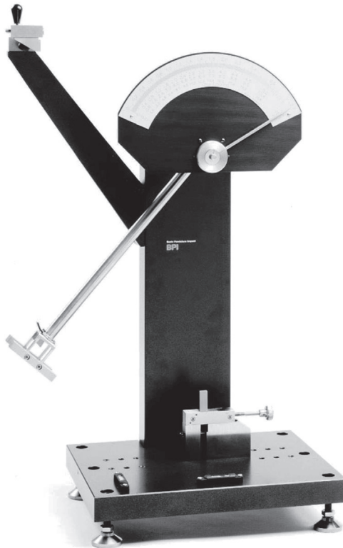
Figure 2.19 Typical analog (noninstrumented) impact testing machine. (Reproduced with permission from Qualitest, www.WorldofTest.com .)
