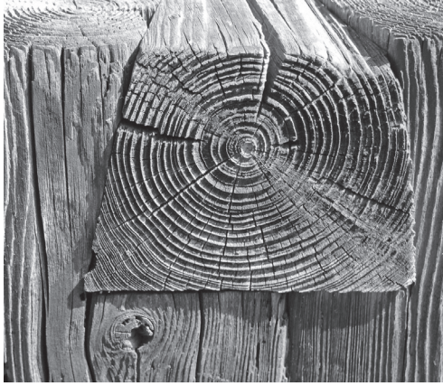
Figure 5.2 The microstructure of wood is typically orthotropic.
