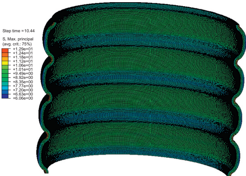
Figure 3.12 Contours of maximum principal stress (in MPa): temperature T = 100\text{ }^\circ\text{C} , P = 120\text{ kPa} , F = 0\text{ N} , loading time t = 60\text{ s} .
