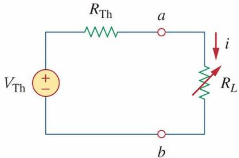
$$i_L = V_{Th} / (R_{Th} + R_L)$$
