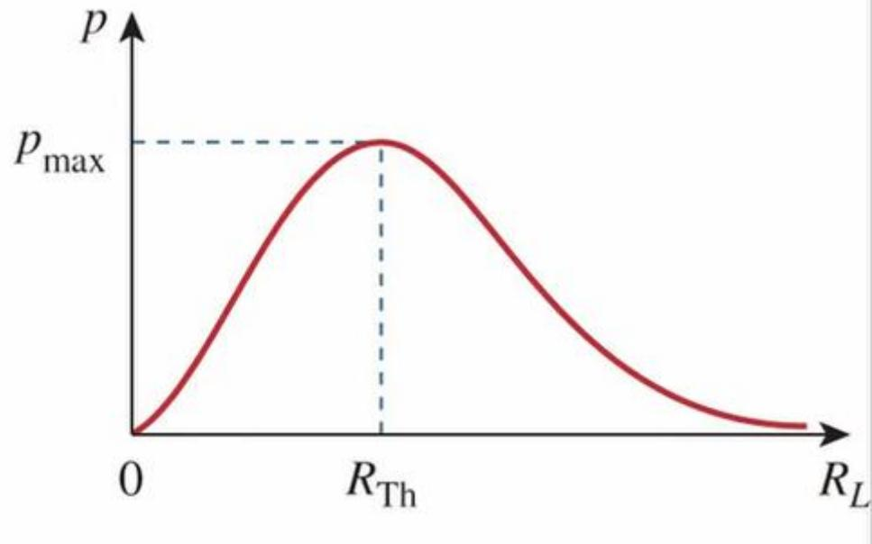
$$\frac{dP}{dR_L} = \frac{V_{th}^2}{(R_{th} + R_L)^4} \left[ \frac{(R_{th} + R_L)^2 - 2R_L(R_{th} + R_L)}{R_L} \right] = 0$$
