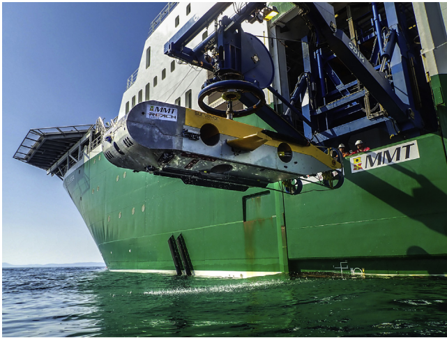
Fig. 17. The 'Surveyor Interceptor' a revolutionary SROV conceived by Ola Oskarsson of MMT to travel between 4 and 6 knots. Chartered to the Black Sea MAP, it carries chirp sub-bottom, multibeam and sidescan sonars as well as HD still cameras synchronised with flash and a laser bathymetry system (Photo: Joakim Holmlund).
