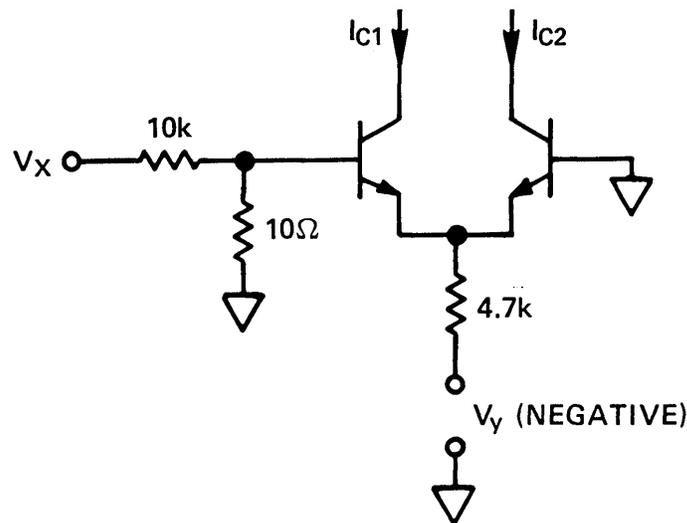
$$I_{c1} - I_{c2} = \Delta I_C = \frac{q}{kT} \left( \frac{V_y + V_{be}}{4.7 \times 10^3} \right) \left( \frac{10}{10,010} \right) V_x$$
