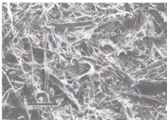
Fig. 16-7. Spruce thermomechanical pulp. SEM micrograph.
