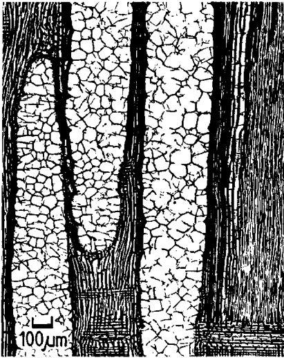
Fig. 2–23. Radial section of robinia ( Robinia pseudoacacia ). The three vessels are filled out with tyloses. Light micrograph (by courtesy of D. Grosser).
