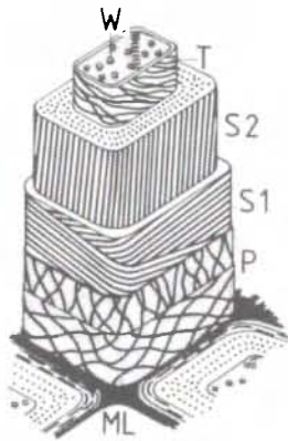
Fig. 2-14. Model of the cell wall structure of softwood tracheids and hardwood libriform fibres. ML = middle lamella, P = primary wall, S 1 = secondary wall 1, S 2 = secondary wall 2, T = tertiary wall, W = wart layer.
