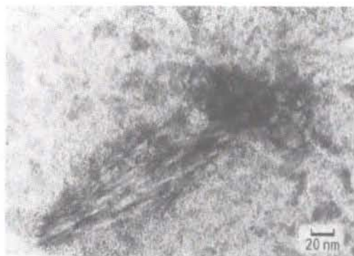
Fig. 17-24. Loose cellulose bundle and molecular cords of methylcellulose from a highly dilute solution. Negative staining, TEM micrograph.
