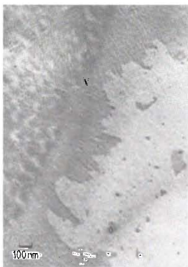
Fig. 12–8. Cellulose isolated from spruce wood heated at 200 °C for 24 hours. Suspension from buffer solution, TEM micrograph.
