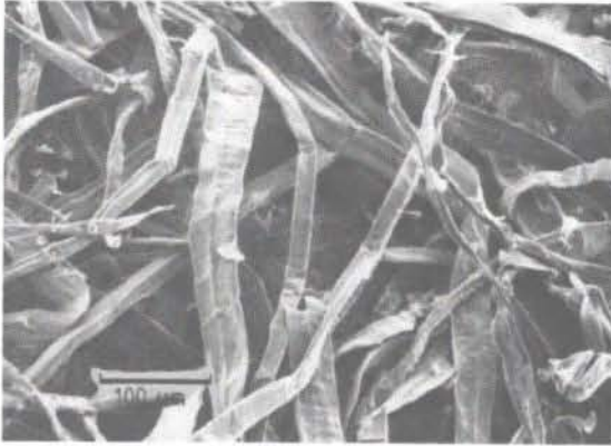
Fig. 16–18. Unbleached spruce sulfite pulp. SEM micrograph.
