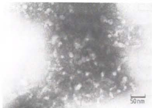
Fig. 17–26. Coiled Na-CMC molecules from a highly dilute solution. Negative staining, TEM micrograph.
