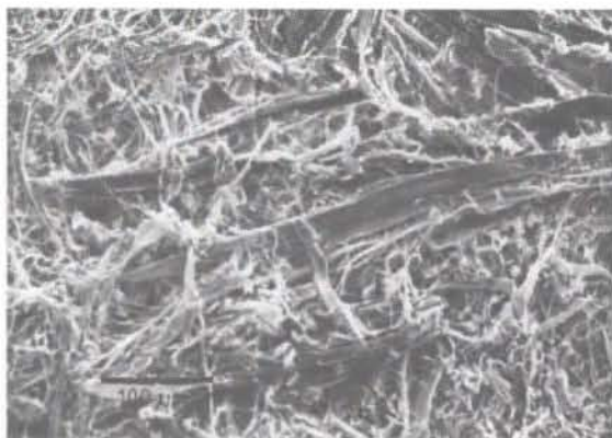
Fig. 16-5. Bleached groundwood pulp. SEM micrograph.
