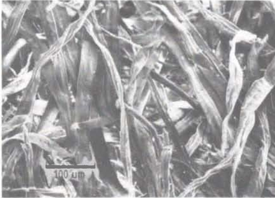
Fig. 16–13. Unbleached pine kraft pulp. SEM micrograph.
