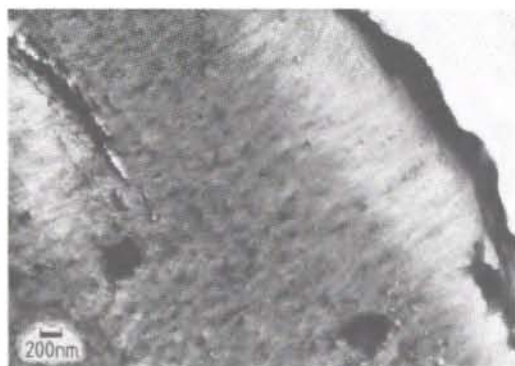
Fig. 8-3. Ultrathin cryo-section of a tracheid wall of spruce ( Picea abies ) in swollen state after delignification and alkali extraction. Places of previously high polyose concentration are more intensively stained. TEM micrograph.
