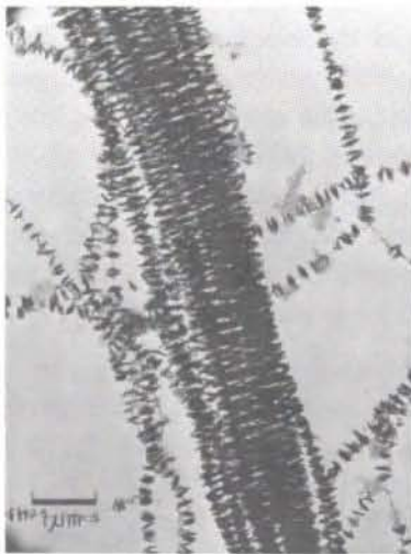
Fig. 5-11. Ivory nut mannan recrystallized on cellulose fibrils forming a shish-kebab structure. Electron micrograph (by courtesy of H. Chanzy).
