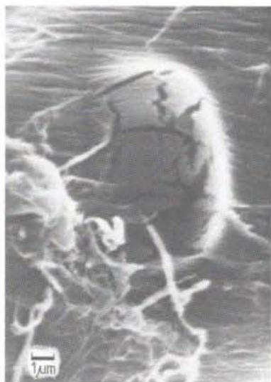
Fig. 12–16. Formation of a bubble and disappearance of the fibrillar structure on the surface of a cotton fibre after exposure to a high-energy electron beam. REM micrograph.
