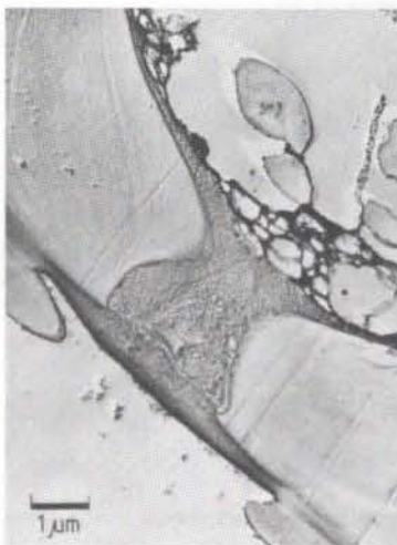
Fig. 5-14. Fibrillar callose seals a half-bordered pit at the parenchymatous side. Ultrathin section of beech wood, electron micrograph.
