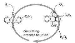
Figure 11.11. Anthraquinone is first reacting with hydrogen and then oxidized with air (oxygen) which forms hydrogen peroxide as a free molecule. (Kemira Kemi).
