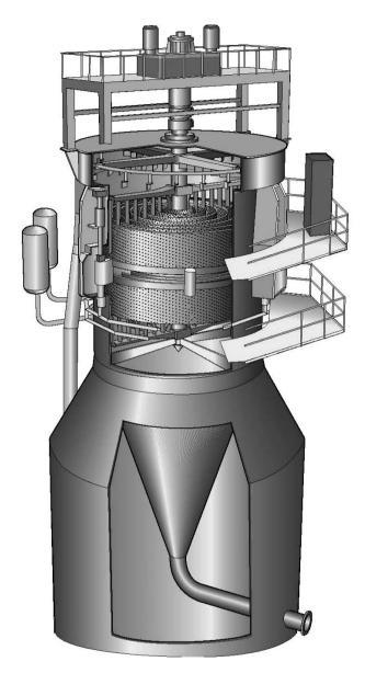
Figure 8.17. Double atmospheric diffuser on top of a pulp storage tank. (Kvaerner Pulping)
