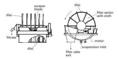
Figure 13.6. Schematic diagram of a rotary filter.
