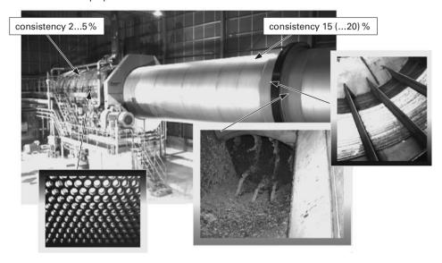
**Figure 15.19.** The FibreFlow<sup>®</sup> drum pulper (Andritz-Ahlstrom<sup>™</sup>) above is common as pulping equipment when repulping recycled paper for production of DIP for news and magazines.
