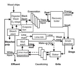
**Figure 14.10.** Purging media for NPEs in a kraft pulp mill. The liquor cycle is represented with solid lines, and the lime cycle with dashed lines. The red dotted lines represent a proposed concept for the recycle of bleach plant filtrate.
