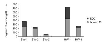
**Figure 9.39.** Totally bound organic chlorine (Bound Cl) and extractable organic chlorine (EOCl) in softwood and hardwood (birch) kraft pulps. Bleaching sequences: SW 1 = (C85+D15)EDED, SW 2 = O(C85+D15)(E+P)DED, SW 3 = OZEDP, HW 1 = O(C85+D15)(E+P)DD, HW 2 = OD(E+P)DD (Björklund Jansson et al 1991).
