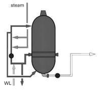
**Figure 6.6.** Circulation of cooking liquor for heating. After the hot liquor fill, the content of the digester is very near of the required cooking temperature. Only a small amount of steam for heating is therefore required and there is no need for expensive heat exchangers, instead a compact direct steam heater can be used. (Metso Paper<sup>©</sup>).
