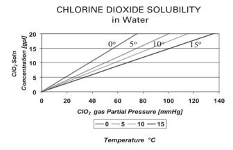
Figure 11.8. The concentration of the chlorine dioxide solution versus the chlorine dioxide partial pressure at  $0-15^{\circ}$ C. (Eka Chemicals, Cellchem).
