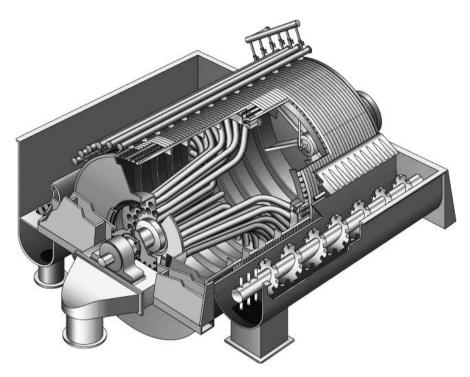
Figure 8.13. Drum filter with filtrate handling. (GL&V).
