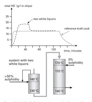
**Figure 7.15.** Split alkali charge using two white liquors is favourable as a high hydrogen sulphide ion concentration is obtained in the beginning of the cook. Split alkali charge using only one white liquor would result in a lower hydrogen sulphide concentration at the beginning.
