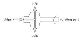
Figure 1.3. A chip refiner with one rotating disc.
