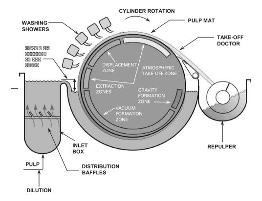
Figure 8.10. Working principle of drum filter. (GL&V).
