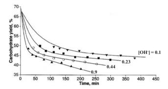
**Figure 7.4.** The loss of carbohydrate yield at different hydroxide ion concentration. Observe that the liquor composition is assumed constant during the cook. (Lindgren 1997).
