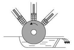
Figure 1.2. A schematic figure of a stone grinder.
