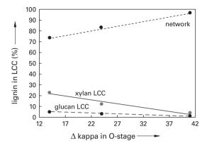
**Figure 9.17.** Amount of lignin chemically linked to glucan, xylan and xylan-glucomannan (network) respectively in softwood kraft pulp after an O-stage. The conditions in the O-stage was adjusted to obtain a range of pulps having different degrees of delignification. The amount of non-linked lignin was zero (Lawoko 2005).
