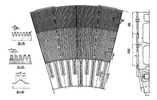
Figure 4.21. Refiner segment. Measure in mm.
