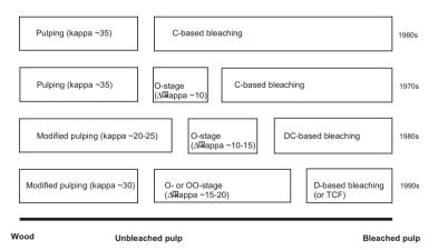
**Figure 9.5.** Schematic illustration of the development of pulping and bleaching technologies for softwood kraft pulp (Rööst 2004).
