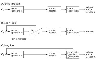
Figure 11.18. Ways to reuse oxygen in connection to ozone bleaching.
