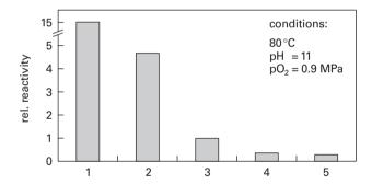
Figure 9.12. Relative reactivities of lignin model compounds on oxidation with oxygen/alkali. 1 = diguaiacylstil-bene, 2 = enol ether from β-O-4 structure, 3 = propylguaiacol, 4 = phenolic β-O-4 structure, 5 = 5,5°-bis-propylguaiacol (Johansson 1997).
