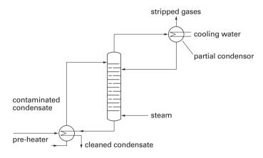
Figure 12.14. Schematic drawing of the condensate column.
