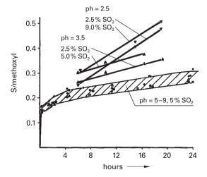
Figure 5.36. Degree of lignin sulphonation after sulphite cooks of spruce wood at various pH-values and charges of sulphur dioxide as a function of time at 135 °C. (Lindgren 1952)
