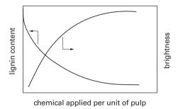
Figure 10.3. The general behaviour of brightness increase and lignin degradation in a given bleaching stage versus the amount of chemicals applied.
