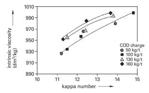
**Figure 10.13.** The viscosity at a given kappa number after oxygen delignification is increased if the unbleached pulp contains increasing amounts of oxidized COD i.e. dissolved organic material that has already been oxidized in the oxygen stage and then recycled. The same pulp as in Figure 10.12. (Metso Paper).
