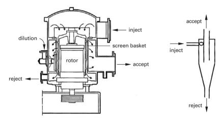
Figure 4.26. Principal sketch of a screen and a Vortex cleaner.
