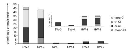
**Figure 9.38.** Presence of chlorinated phenols (gram/tonne) in bleached kraft mill effluents. SW = softwood, HW = hardwood. Bleaching sequences: SW-1 = O(C92+D8) (EO)DED; SW-2 = O(D25, C70+D5)(EPO)D(EP)D; SW-3 = OD(EPO)D(EP)D; SW-4 = OD(EO)D(EP)D; HW-1 = (D80+C20)(EPO)DED; HW-2 = O(D27, C68+D5)(EPO)D(EP)D. (Strömberg et al 1996).
