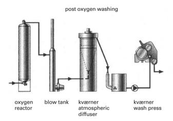
Figure 8.29. Washing after oxygen delignification. (Kvaerner Pulping).
