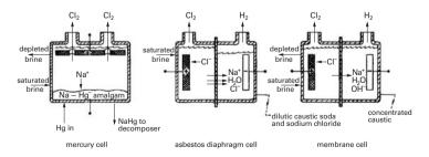
**Figure 11.9.** Three different types of electrolysis cells for production of chlorine and alkali (Olin Corporation).
