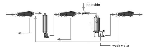
Figure 10.38. A two-stage MC/HC peroxide stage. (Metso Paper).
