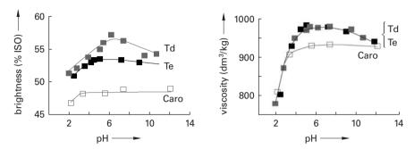
**Figure 10.24.** Influence of pH in a peracetic acid stage and a Caro's acid stage.  $T_{\rm d}$  denotes distilled peracetic acid and  $T_{\rm e}$  denotes peracetic acid in equilibrium with hydrogen peroxide and acetic acid. (Eka Chemicals).
