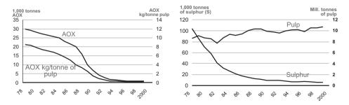
**Figure 14.5.** The emissions of AOX to water and sulphur to air have been decimated during the last two decades.
