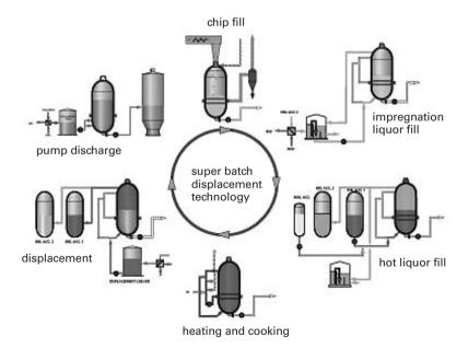
**Figure 7.14.** The SuperBatch system. The black liquor displaced after the cook is first used in the hot liquor fill. After displacement from that stage it is used in the impregnation. Finally, after displacement from the impregnation stage the black liquor goes to evaporation and recovery furnace. The white liquor is added at the later part of the hot liquor fill. (Metso Paper<sup>©</sup>).
