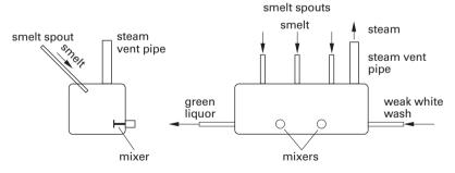
Figure 13.3. The smelt dissolver from two perspectives.
