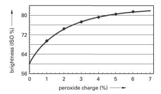
**Figure 10.32.** The brightness of a TMP pulp versus the peroxide charge. Bleaching conditions used: 3 hours, 70 °C, 3 % silicate, 25% consistency, Spruce TMP, 60% ISO (Metso Paper).
