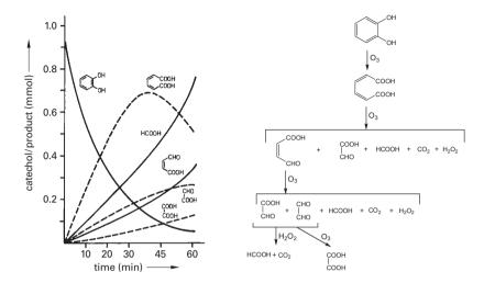
Figure 9.41. Ozonation of catechol in water at 30 °C. Formation of products as a function of ozonation time (left) and suggested mode of formation of products (right). (Yamamoto et al 1979.)
