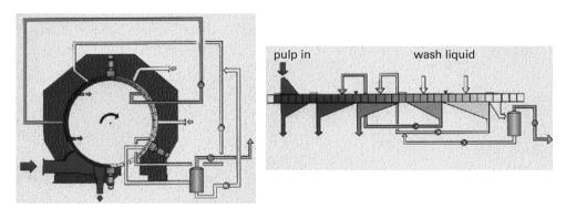
Figure 8.23. Operating principle for a 2-stage DD-washer. (Andritz).
