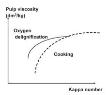
Figure 10.8. The pulp viscosity versus the kappa number for oxygen and non-oxygen delignified pulps.
