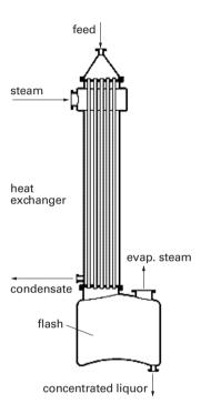
Figure 12.7. Schematic diagram of a fallingfilm evaporator.
