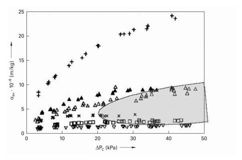
Figure 13.16. Specific filtration resistance versus pressure for 8 different mills in Sweden.
