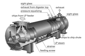
Figure 6.12. Steaming vessel (Kvaerner Pulping).
