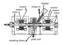
Figure 4.2. Double disc refiner.
