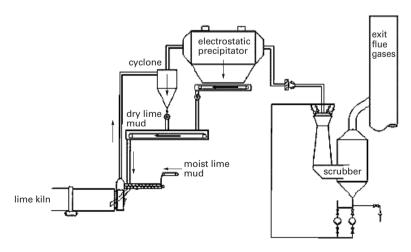
Figure 13.23. Lime kiln with a separate section for drying lime mud.
