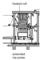
Figure 1.9. The extended nip makes the press section more efficient.
