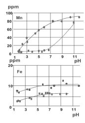
**Figure 10.22.** The influence of pH on the content of manganese, magnesium and iron ions in softwood kraft pulps without EDTA or with or 2 kg EDTA/t. (Eka Chemicals).
