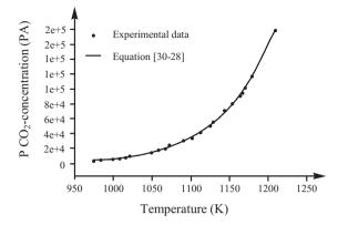
Figure 13.19. Equilibrium concentration of carbon dioxide versus temperature.
