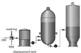
**Figure 6.8.** Discharge of the pulp, also denoted blow, as the pulp is admitted from the pressure within digester to atmospheric pressure in the flash tank. (Metso Paper<sup>©</sup>).
