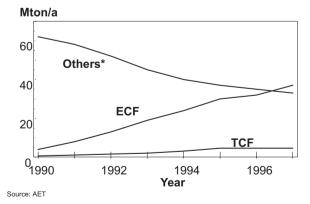
**Figure 10.14.** The world trend concerning bleaching with sequences including chlorine gas (others), chlorine dioxide but not chlorine gas or hypochlorite (ECF) or neither chlorine gas, chlorine dioxide or hypochlorite (TCF).
