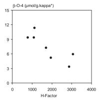
Figure 5.33. Remaining amount of  $\beta$ -O-4 structures in the residual lignin of softwood kraft pulp as a function of the H-factor. Pulping to a kappa number of 20 after correction for the contribution from hexenuronic acid using various charges of hydroxide and hydrosulphide ions. Analysis by thioacidolysis.
