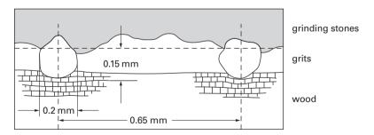
Figure 4.18. Typical dimensions of the surface of a grinding stone. The grits treat the fibres perpendicular to their longitudinal axis.
