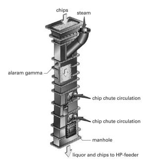
Figure 6.13. Chip chute (Kvaerner Pulping).
