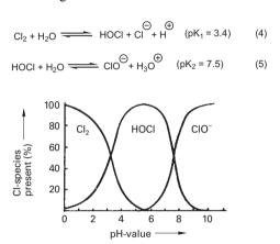
Figure 9.26. Chlorine species present in aqueous solution (room temperature) at different pH-values.
