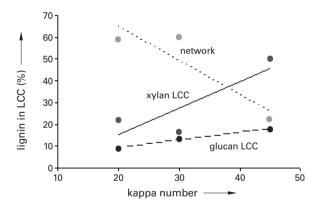
**Figure 9.4.** Amount of lignin chemically linked to glucan, xylan and glucomannan-xylan (network) respectively in softwood kraft pulps having different kappa numbers. The amount of non-linked lignin is  $\sim 10\%$  of the total (Lawoko 2005).
