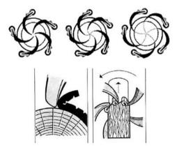
**Figure 2.9.** The barking technique performed by the one-log barker. The log is held by the spiked rolls and transported forward, while the barking tools rotate and shave off the bark (Copyright Söderhamn, Eriksson and Cambio).
