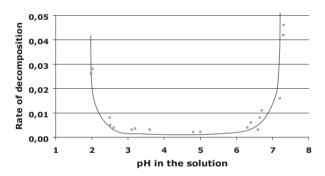
Figure 11.13. The rate of decomposition of a hydrogen peroxide solution is lowest between pH 4 and 5. (Kemira Kemi).
