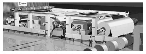
Figure 1.10. Paper wound onto reels and subsequently cut to suitable width (Metso Paper).
