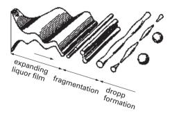
Figure 12.24. Schematic description of the drop formation mechanism.
