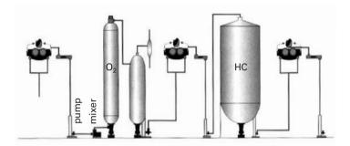
**Figure 10.10.** A medium consistency oxygen delignification stage consisting of a wash press, a transportation screw, a stand-pipe with a pump, a mixer and a reactor with a following blow tank, a wash press, a HC tower (buffer tank) and a final wash press. (Metso Paper).
