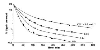
**Figure 6.29.** The bulk and residual delignification in cooks conducted at different concentration of hydroxide ions. [HS<sup>-</sup>] = 0.28 mol/l, temp = 170 °C. (Lindgren and Lindström 1996).
