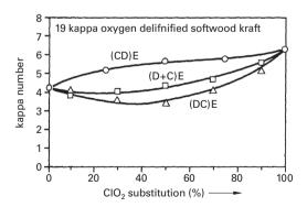
**Figure 10.16.** The kappa number after (CD)E, (C+D)E and (DC)E prebleaching of an oxygen delignified softwood kraft pulp versus the chlorine dioxide substitution. The same active chlorine charge was used in all cases. (Axegård 1986).
