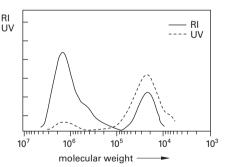
**Figure 5.34.** GPC analysis of unbleached kraft pulp from pine (left) and birch (right) after dissolution in dimethylacetamide/lithium chloride. RI = refractive index, UV = ultraviolet detection. Molecular weight calibration with pullulan standards. (Karlsson 1997).
