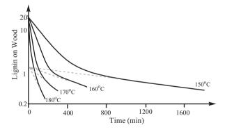
**Figure 6.33.** Delignification rate affected by varied cooking temperature.  $[OH^-]=0.44 \text{ mol/l}$ ,  $[HS^-]=0.44 \text{ mol/l}$  (Lindgren and Lindström 1996).
