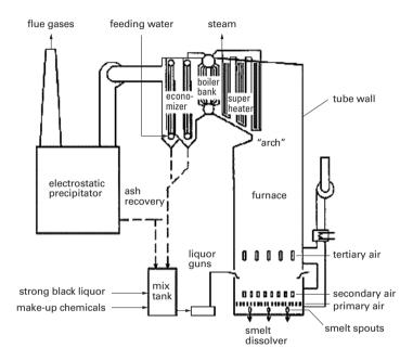
Figure 12.16. A schematic diagram of the recovery boiler.
