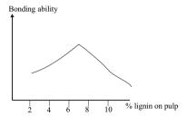
**Figure 16.21.** Lignin on the fibre surface prevents good bonding between fibres and hemicelluloses promote it. At a certain point, the lignin on the surface has been removed and further delignification dissolves hemicelluloses and the bonding ability starts decreasing.
