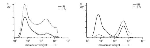
**Figure 9.3.** GPC-analysis of unbleached kraft pulp from pine (left) and birch (right) after dissolution in dimethylacetamide/lithium chloride. RI = refractive index, UV = ultraviolet detection. Molecular weight calibration with pullulan standards. (Karlsson 1997).
