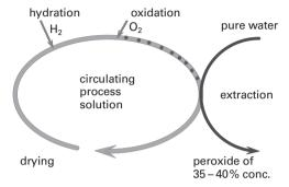
Figure 11.10. A simplified description of the hydrogen peroxide production process. (Kemira Kemi).
