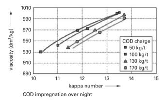
**Figure 10.12.** The viscosity at a given kappa number after oxygen delignification is decreased if the unbleached pulp contains more unoxidized COD i.e. more dissolved organic material from the digester. Softwood kraft pulp. (Metso Paper).
