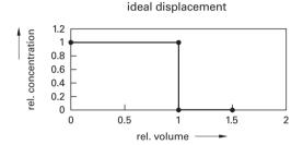
Figure 8.5. Ideal displacement or an infinite number of stages.
