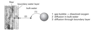
Figure 9.6. Schematic view of the transfer of oxygen from the gaseous phase to the reaction sites in the fiber wall.
