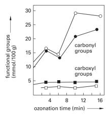
Figure 9.44. Formation of carbonyl and carboxyl groups in unbleached softwood kraft pulp (filled symbols) and in  $\alpha$ -cellulose (unfilled symbols) as a function of ozonation time at 23 °C. (Chandra and Gratzl 1985.)
