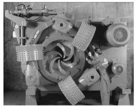
Figure 2.8. One-log barker used primarily in sawmills (Copyright Söderhamn Eriksson Cambio).
