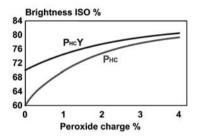
**Figure 10.39.** The brightness obtained after an HC-peroxide stage and a MC-hydrosulphite stage or after a single HC-peroxide stage. Bleaching conditions used: 0.8% hydrosulphite, Spruce TMP, 60 % ISO (Metso Paper).
