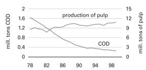
**Figure 10.30.** The discharge of COD from the Swedish pulp mills has decreased by more than 85 % between 1978 and 2000 while at the same time the pulp production has increased from 9 to 11 million ton/a. (The Swedish Forest Industries Federation).
