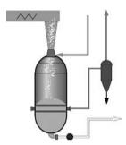
Figure 6.3. Chip filling of batch digester. (Metso Paper<sup>©</sup>).
