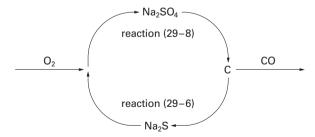
Figure 12.20. The sulfate/sulfide cycle.
