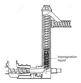
Figure 4.30. Chip impregnator.
