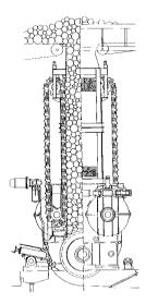
Figure 4.17a. The principle of the Voit chain ginder.
