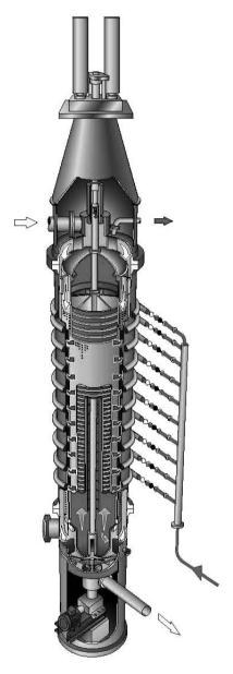
Figure 8.18. Pressure diffuser. (Kvaerner Pulping).
