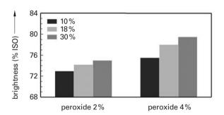
**Figure 10.36.** Pulp brightness for hydrogen peroxide bleaching with 2 or 4% and at different pulp consistencies. Bleaching conditions used: 3 hours, 70 °C, 3% silicate, Spruce TMP, 60% ISO (Metso Paper).
