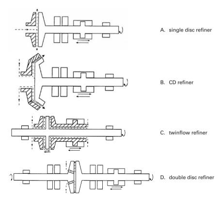
Figure 4.22. Different types of chip refiners.
