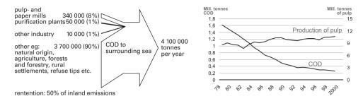
**Figure 14.4.** The share of the Swedish emissions of oxygen-demanding substances (COD) emanating from the pulp and paper industry has declined as a result of process improvements, reduced water consumption and effluent treatment.
