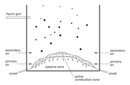
Figure 12.21. A schematic figure of the lower part of the furnace.
