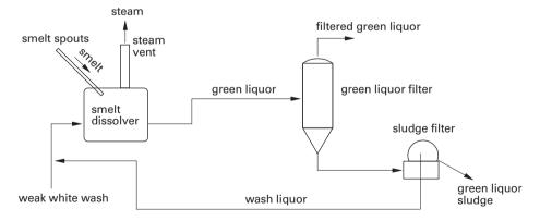
Figure 13.2. Schematic diagram of the green liquor system.
