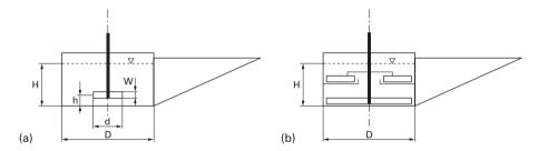
Figure 13.10. Different types of slakers.
