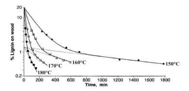
**Figure 7.9.** Temperature has no effect on the relative amount of bulk phase lignin and residual phase lignin. (Lindgren and Lindström 1996).
