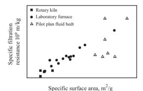
Figure 13.17. Specific filtration resistance of lime mud versus specific surface area of reburned lime mud.
