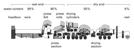
Figure 1.7. A simplified plot of a paper machine.
