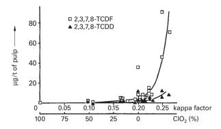
**Figure 9.37.** Sum of 2,3,7,8-TCDF and 2,3,7,8-TCDD in bleached softwood kraft pulp as a function of the charge of active chlorine in the pre-bleaching stage. (Axegård and Renberg 1989).
