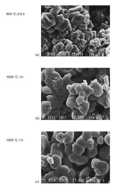
**Figure 13.20.** Examples of lime mud calcined under different conditions: a) 900 °C 0.5 h, b) 1100 °C 1h, c) 1300 °C 1h.
