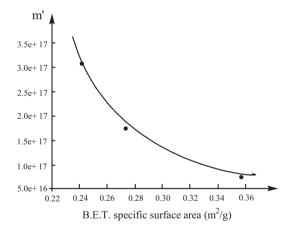
Figure 13.14. The parameter m' versus the specific surface area of the reburned lime mud.
