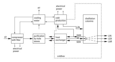
Figure 11.1. An overview of the conventional oxygen production process using air distillation also called cryogenic distillation. (Aga Linde Gas).
