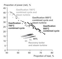
**Figure 14.15.** The division of the energy content in the black liquor between power and heat for different pressurized black liquor gasification alternatives. Recovery boilers with different steam data points and black liquor solids content are included as a comparison.
