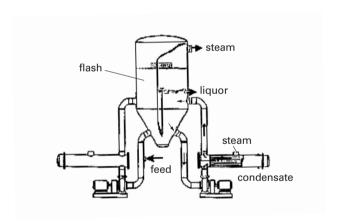
Figure 12.6. Diagram of a forced circulation evaporator designed for crystallisation.
