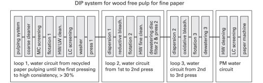
**Figure 15.10.** Advanced process concept for fine paper grades (high grade printing and writing papers) or market pulp based on Mixed Office Waste (MOW). What is not shown in the process concept is the rejects from screening, cleaning, flotation and washing steps, in total somewhere between 30 and 35 % of the incoming recycled paper.
