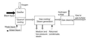
**Figure 14.14.** Chemical and energy recovery with pressurized black liquor gasification. Generated hydrogen sulphide can be converted to sulphuric acid and polysulphide via Sulphur production in the Claus Process.
