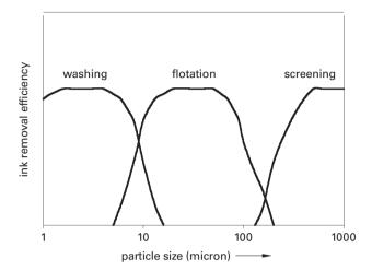
**Figure 15.7.** The removal of contaminants using various separation techniques. The importance of the particles size on the separation process and the efficient size intervals for the different separation techniques.
