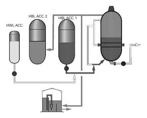
Figure 6.5. Hot liquor fill. HWL = hot white liquor, HBL = hot black liquor. (Metso Paper<sup>©</sup>).
