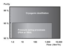
**Figure 11.3.** The purity of the delivered oxygen versus the production capacity given as m<sup>3</sup> oxygen per hour. Onsite production with PSA or VSA and off-site cryogenic distillation are shown. Note that the flow scale is logarithmic (Aga Linde Gas).
