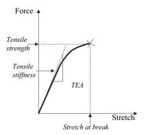
Figure 16.13. The stress-strain curve for tensile strength testing.
