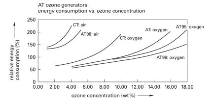
**Figure 11.15.** The power consumption in ozone generation versus the ozone gas concentration for air and oxygen. The figure shows that the power demand has been decreased during the 1990's. (Ozonia).
