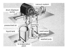
Figure 8.24. A DD-washer and schematic system (Andritz).
