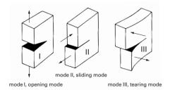
Figure 16.14. Tearing forces applied in different modes. (Illustration STFI).
