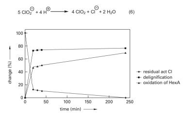
**Figure 9.30.** Oxidation of an oxygen delignified eucalyptus kraft pulp (kappa number 10.4) with 2.08 % chlorine dioxide (as active chlorine) at pH=3.0 and 60 °C. Separate analyses of lignin oxidation (delignification) and hexenuronic acid (HexA) oxidation.
