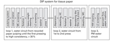
**Figure 15.11.** Typical process concept for tissue paper grades normally based on both Mixed Office Waste (MOW) and household collection of old news and old magazines (ONP / OMG). What is not shown in the process concept are the rejects from screening, cleaning, flotation and washing steps, in total somewhere between 30 and 37 % of the incoming recycled paper.
