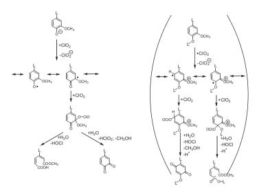
**Figure 9.25.** Reactions between a phenolic (left) and a non-phenolic (right) lignin structure respectively with chlorine dioxide under acidic conditions (Eriksson 1993). In benzylalcohol structures, a similar reaction will result in an oxidative elimination of the side chain. The reaction of non-phenolic lignin structures is less likely under technical pre-bleaching conditions.
