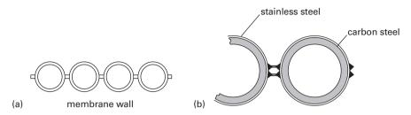
Figure 12.31. Tubes in the furnace.
