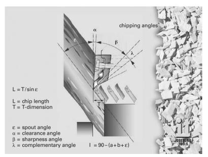
Figure 2.13. Chipper geometry. The angles vary with different chipper manufacturers, the β-angle usually is between 32° and 38°, the α-angle between 2° and 4°, and the  $\varepsilon$ -angle is typically 32–38° (Iggesund Tools<sup>©</sup>).
