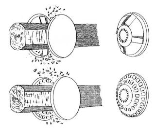
**Figure 2.20.** Two types of reducers used in sawmills. Above a long-knife disc, cutting chips across the fibre direction. Below a spiral disc, cutting chips parallel to fibre direction.
