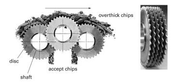
Figure 2.25. Disc screen used separation of the overthich chips. (Acrowood<sup>©</sup>)
