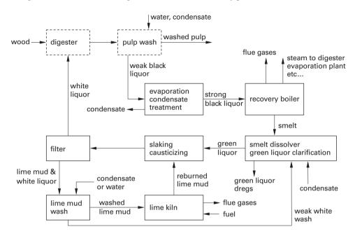
Figure 12.1 is a schematic diagram of the chemical recovery plant.
