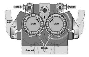
Figure 8.22. The "Compact Press". (Kvaerner Pulping).
