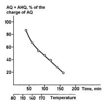
Figure 5.26. Consumption of anthraquinone (AQ) and anthrahydroquinone (AHQ) in soda-AQ pulping. (data from Kubes et al 1980).
