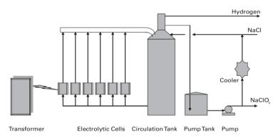
Figure 11.4. Sodium chlorate production via electrolysis of sodium chloride (Eka Chemicals, Cellchem).
