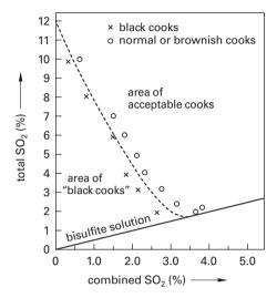
Figure 5.35. Influence of the sulphite pulping liquor composition on the formation of lignin condensation reactions ("black cooks"). Charge of sulphur dioxide/bisulphite in per cent on wood. (Kaufmann 1951).
