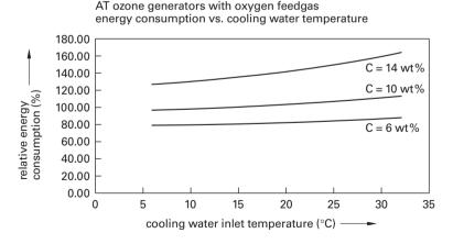
**Figure 11.16.** The relative ozone consumption versus the cooling water temperature with the ozone gas concentration as parameter. (Ozonia).
