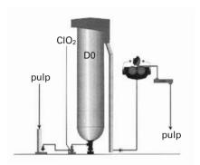
**Figure 10.1.** A bleaching stage of up-flow type. There is no over pressure at the top of the reactor and the reactor is denoted as atmospheric. The stage is of medium consistency type. (Metso Paper).
