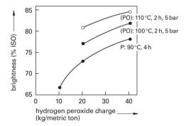
**Figure 10.23.** Bleaching with P and (PO)-stages shows that a higher brightness is obtained after a (PO)-stage. (Metso Paper).
