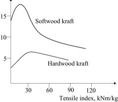
**Figure 16.15.** The refining energy input is varied for a softwood kraft pulp and a hardwood kraft pulp and the pulps tear and tensile strengths are recorded. Prolonged beating increases tensile strength whereas tear strength decreases.
