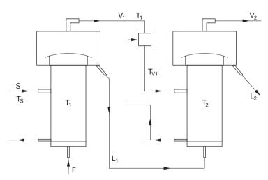
Figure 12.12. Saturating superheated steam by injection with saturated condensate.
