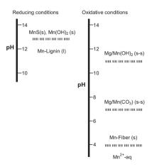
**Figure 9.16.** Possible manganese(II) compounds under reducing (pulping) and oxidative (O-stage) conditions respectively. s = solid; l = soluble complex; s-s = solid solution (Lidén 1994.)
