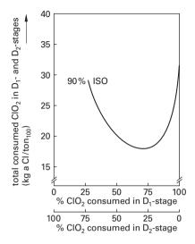
**Figure 10.19.** The split of chlorine dioxide between the  $D_1$  and the  $D_2$ -stages when bleaching to full brightness. (Axegård, Jansson, Teder 1984).
