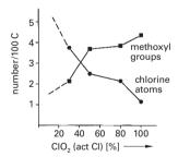
**Figure 9.31.** Composition of the dissolved lignin (from E-stage) after pre-bleaching of softwood kraft pulp with different ratios of Cl/ClO<sub>2</sub>. Degree of oxidation measured as number of methoxyl groups/100 carbon atoms and degree of chlorination as number of Cl/100 carbon atoms.
