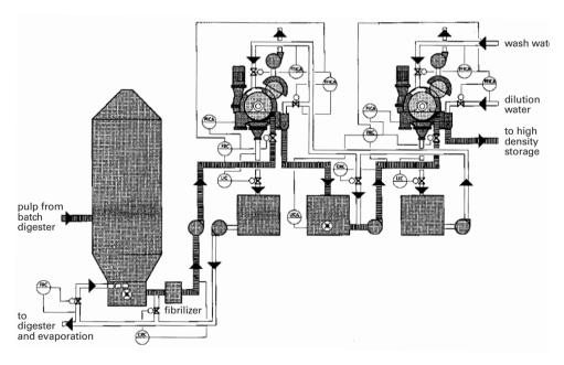
Figure 8.40. Schematic PID for a washing plant.
