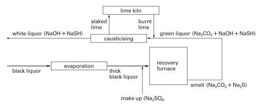
Figure 1.6. The stages in recovery of chemicals and energy in the kraft process.
