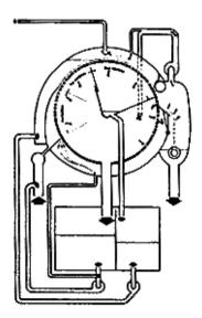
Figure 8.14. The principle for a two-stage pressure washer. (Metso Paper).
