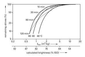
**Figure 10.27.** Calculated percentage of remaining shives versus calculated chromophore content in the pulp fibres of an O(C + D)E-prebleached pulp after bleaching with chlorine dioxide at different temperatures. The pH and the chlorine dioxide concentrations were kept constant. Reaction times are given as broken lines. (Axegård 1979).
