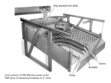
**Figure 2.24.** Chip screen with perforated plates shaking the chips to achieve separation of oversize chips, pin chips and fines from accept chips (Metso Paper<sup>©</sup>).
