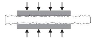
Figure 16.16. Thickness, or caliper, gauge according to SCAN standard.
