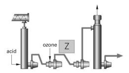
**Figure 10.20.** A medium consistency ozone stage consisting of a stand-pipe with an MC-mixer, two mixers in series and a final standpipe with separation of the residual gases. (Kvaerner Pulping).
