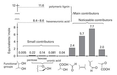
**Figure 5.31.** Consumption of acidic potassium permanganate (equivalents/mole) in the oxidation of various structures/functional groups. Reaction conditions identical to those used in the standard kappa number measurement.
