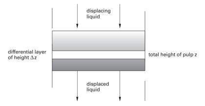
Figure 8.2. A model for the displacement process.
