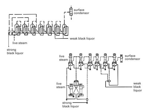
Figure 12.2. Schematic diagram of some typical black liquor evaporation plants.
