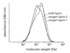
**Figure 9.10.** Gel permeation chromatography of lignins dissolved from a kraft cook and from a subsequent O-stage respectively. Delignification in the O-stage was around 8 (lignin 1) and 15 (lignin 2) kappa number units respectively. Molecular weight calibration with polystyrene standards.
