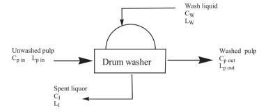
Figure 8.7. A single Washing Stage (Drum Washer).
