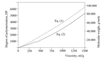
**Figure 16.6.** Degree of polymerisation and molecular weight vs. SCAN viscosity. Curvature according to Equation 1 is suggested by Evans and Wallis (1987) and Equation 2 by Marx Figini (1978) and Gruber (1981).
