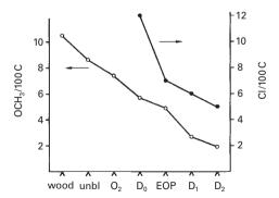
**Figure 9.28.** Changes in methoxyl and chlorine content in the residual lignin of industrial softwood kraft pulp when going from wood to fully bleached pulp. Bleaching with the sequence OD(EOP)DD. Number of methoxyl groups per 100 carbon atoms and chlorine atoms per 1000 carbon atoms.
