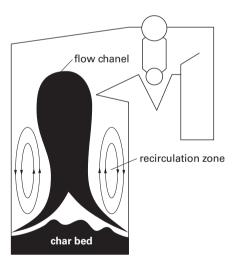
Figure 12.27. Channeling caused by a high flow rate of the primary air.
