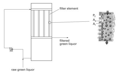
Figure 13.7. Schematic diagram of a so-called "X-filter".
