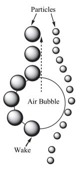
**Figure 15.14.** The reason to why small particles do not flotate. Small particles follow the stream lines around a rising bubble and therefore do not collide with the bubble. The momentum of the particle is to low. A larger particle on the other hand collides and can therefore attach if the interactions between the particle and the bubble are favourable.
