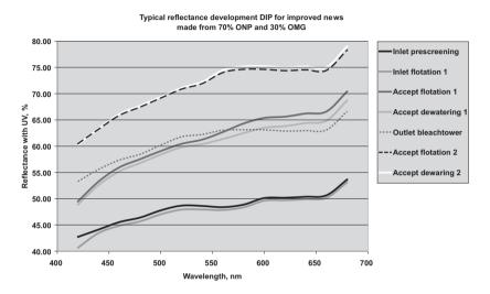
**Figure 15.9.** Normally only the brightness around 457 nm (ISO brightness), or 557 nm (Y-value) are measured. This figure however describes typical reflectance spectra along the whole visible spectrum measured on lab sheets (P. Engstrand).
