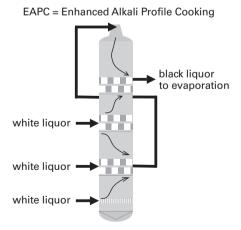
Figure 7.13. Black liquor impregnation is included in the EAPC process.
