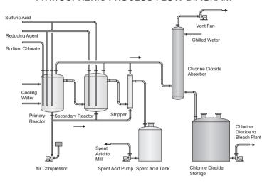
**Figure 11.6.** An atmospheric chlorine dioxide generator with primary and secondary reactor, stripper, absorption tower and chlorine dioxide storage tank. The process type is HP-A process where hydrogen peroxide is used as the reducing agent. The old Mathieson process is similar if the hydrogen peroxide is replaced with sulphuric dioxide (Eka Chemicals, Cellchem).
