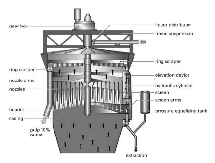
Figure 8.16. Principle of an atmospheric diffuser. (Kvaerner Pulping).
