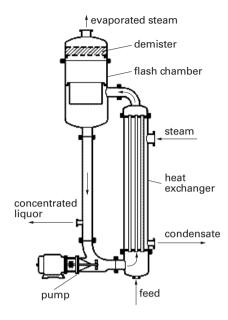
Figure 12.5. Diagram of a forced circulation evaporator.
