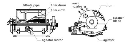
Figure 13.18. Schematic diagram of a rotary drum filter.
