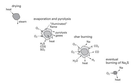
Figure 12.18. Schematic diagram of the four operations.
