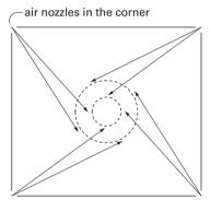
Figure 12.29. An alternative way of mounting the nozzles at the tertiary air level.
