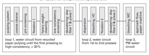
**Figure 15.8.** Typical process concept for newsprint and improved news. Typical data; 40–90 g/m² papers, yield approximately 83 %, effluent approximately 8 m³/t, filler; feed 22 % finished paper 13 %, brightness 63–66 %ISO. What is not shown in the process concept are the rejects from screening, cleaning and flotation, in total somewhere between 15 and 25 % of the incoming recycled paper.
