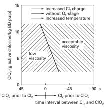
**Figure 10.15.** The figure shows that if a low charge of chlorine dioxide is used in a chlorine stage to protect the pulp viscosity it is best to charge it after the chlorine. (R Grundelius 1979).
