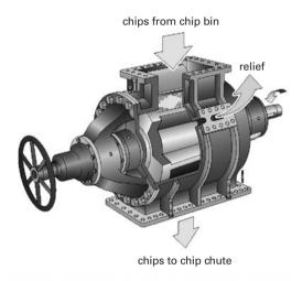
Figure 6.11. LP feeder (Kvaerner Pulping).
