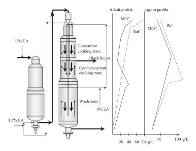
Figure 7.10. MCC -the first of the "new" pulping types based on kinetics.
