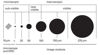
Figure 15.24. The measurement techniques used for ink particles of varying sizes.
