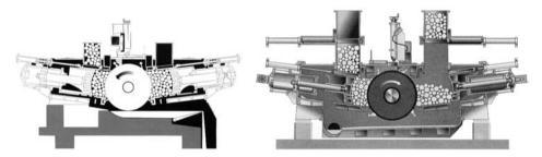
Figur 4.17b. Modern atmosperic Valmet grinder. Figure 4.17c. The Valmet Pressurizedpocket (PGW) grinder.
