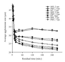
**Figure 13.13.** Example of the disintegration of lime mud agglomerates. Average agglomerate size versus the residence time, impeller type (HFI= high flow impeller, PBT = "Pitched-blade turbine" and RT = "Rushton turbine") and impeller speed.
