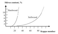
**Figure 6.19.** The defibration point is defined as the kappa number at which the shives content approaches zero. For hardwood, the defibration point is approximately at kappa number 20 and for softwood around 45.
