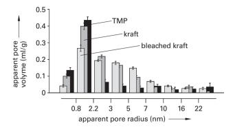
**Figure 5.30.** Apparent pore volume at different pore size intervals for mechanical pulp (TMP), unbleached kraft pulp (kappa 78) and bleached kraft pulp (kappa 0.5) determined by inverse size exclusion chromatography (ISEC). (Berthold 1996).
