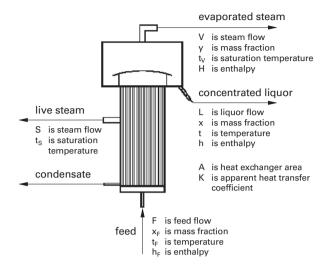
Figure 12.10. Notations used in evaporation calculations.
