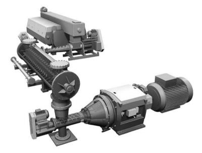
**Figure 15.23.** The picture above describes a typical dispersion system, consisting of a conical plug-screw (in the back) feeding the high consistency DIP to the pressurized pre-heater (up to 120 °C, 3 min residence time) from where the pulp is fed to a feed screw and directly to the disperser, in this case a conical model.
