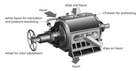
Figure 6.14. HP feeder (Kvaerner Pulping).
