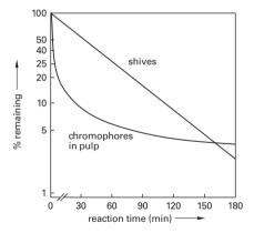
**Figure 10.26.** The figure shows the remaining amount of shives and chromophores in a chlorine dioxide final bleaching stage where the pH and the chlorine dioxide concentrations were kept constant. The different reaction patterns for shives and pulp fibres are obvious. (Axegård 1979).
