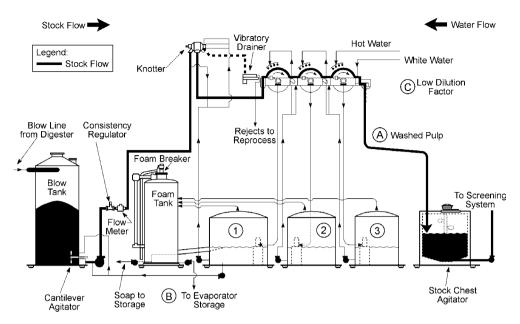
Figure 8.25. Three drum washers in series. (GL&V).
