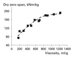
**Figure 16.20.** The viscosity value correlates to the degree of polymerisation of the cellulose chains. Above a certain chain length, the pulp strength is practically unaffected by a decrease in chain length. However, below the critical point, the pulp strength is rapidly reduced with further reduction in viscosity.
