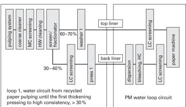
recycled pulp system for packaging paper as test liner
