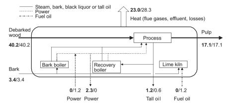
**Figure 14.12.** Thermal energy balance for the reference mill (figures before slash sign), version with bark boiler instead of bark export. As a comparison (figures after slash sign) the average value for Swedish mills that produced market pulp in 1994 is shown. The energy content in the wood and the pulp is given as combustible dry solids. Unit: GJ/ADt.
