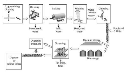
Figure 2.1. Handling of wood at the pulp mill.
