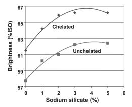
**Figure 10.35.** The effect of the sodium silicate addition on the pulp brightness at optimum alkalinity for chelated (DTPA) and unchelated TMP pulp. Bleaching conditions used: 4 hours, 65 °C, 21% consistency, 3% hydrogen peroxide. (PQ Sweden).
