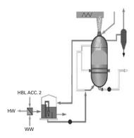
Figure 6.4. Filling of impregnation liquor. (Metso Paper<sup>©</sup>).
