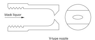
Figure 12.23. Examples of the three nozzles used for the formation of drops.
