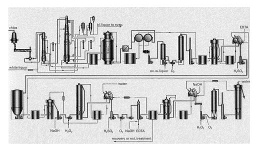
Figure 8.27. A total fibre line based on diffusers and presses (Kvaerner Pulping).
