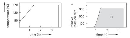
**Figure 6.21.** Left: temperature profile during a cook with heating up period and cooking at 170 °C. Right: The relative reaction rate during the cook. The H-factor is the area under the relative reaction rate curve.
