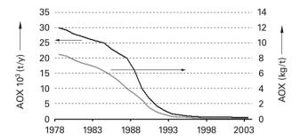
**Figure 9.36.** The decrease of chlorinated organic substances (AOX) from Swedish pulp mills as a function of time. Total amount from all mills in tonnes/year (left) and average value per tonne (right). Source: Skogsindustrierna.
