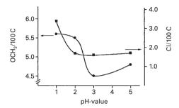
**Figure 9.27.** Oxidation of isolated residual lignin from oxygen delignified softwood kraft pulp with aqueous chlorine dioxide at different constant pH-values. Number of methoxyl groups and chlorine atoms per 100 carbon atoms.
