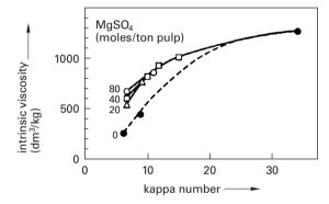
**Figure 10.7.** The addition of magnesium ions to the oxygen stage slurry increases the pulp viscosity at a given kappa number. A softwood kraft pulp was used. (Gustavsson and Swan, 1974).
