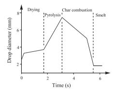
Figure 12.19. An example of swelling and shrinking during the combustion of black liquor.
