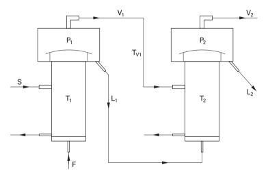
Figure 12.11. A two-unit evaporation plant.
