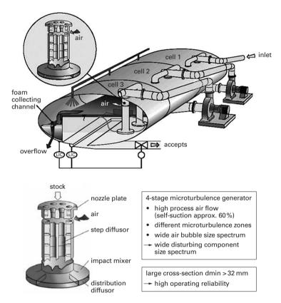
**Figure 15.21.** The flotation equipment above is a modern and very common set-up of Voiths tank flotation system with air injectors in the bottom part of the cells stepwise mixing air into the pulp at 1–1,5 % consistency. The foam created at the surface flows over an edge into a foam channel. In modern systems normally 5–6 steps are used in flotation 1 and 2–3 steps in flotation 2. The injectors consisting of nozzles and step diffusors is also shown.
