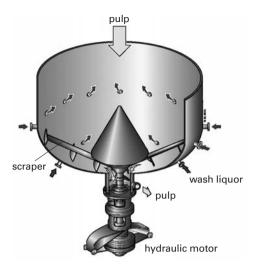
Figure 6.17. The outlet device for digester. (Kvaerner Pulping).
