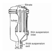
Figure 13.5. An example of a tube filter.
