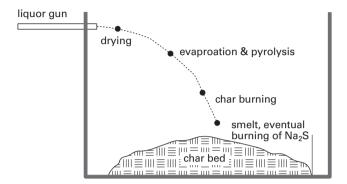
Figure 12.17. Schematic diagram of the route taken by a drop of liquor from the liquor gun to the bed.
