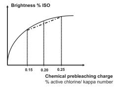
**Figure 10.28.** The figure shows the effect of poor mixing. If 50 % of the pulp gets a too high chemical charge (0.25) and the remaining pulp gets a too low charge (0.15) the average brightness of these two samples is poorer than if the mixing is good and all the pulp gets a homogeneous charge (0.20).
