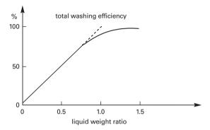
Figure 8.36. Well above 99 % efficiency after expansion with a wash press.
