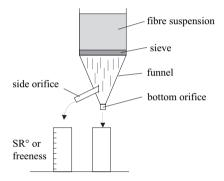
**Figure 16.12.** Drainability test. A fibre suspension is poured into a vessel with a sieve in the bottom. The faster the water drains through the sieve, the higher the water level in the funnel and accordingly more water flows through the side orifice. The water from the side orifice is collected and the amount gives the CSF or SR-number.
