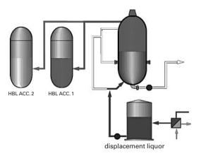
**Figure 6.7.** Displacement of cooking liquor by cool liquor. The hottest cooking liquor is taken to accumulator no. 1 and the warm second part, with lower temperature to accumulator no. 2. (Metso Paper<sup>©</sup>).
