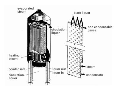
Figure 12.9. Example of an evaporator having plates as the heat exchanger device.
