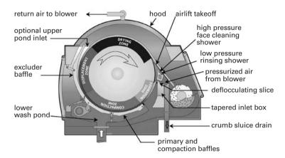
Figure 8.15. CB (Compaction Baffle) filter (GL&V).
