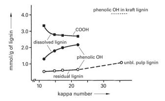
**Figure 9.13.** Amounts (mmol/g of lignin) of carboxyl groups and phenolic hydroxyl groups in lignins after kraft pulping and oxygen delignification respectively. The O-stage was carried out to four different kappa number values by using different charges of alkali in the stage.
