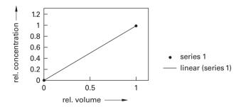
Figure 8.6. The ideal displacement in integrated form as recovery of the solute under consideration.
