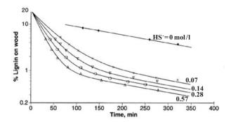
Figure 6.32. The effect of hydrogen sulphide ion concentration on the delignification rate.  $[OH^-] = 0.44 \text{ mol/l}$ , temp = 170°C. (Lindgren and Lindström 1996).
