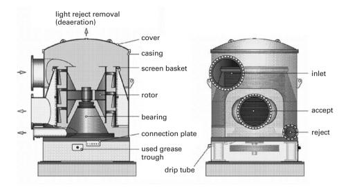
**Figure 15.20.** The screen above is a modern version of screens from Voith Paper a so-called MultiScreen<sup>™</sup> MSS. This is in recycled fibre processes used for combined mostly for fine-screening at low consistency. The same type of screen can also be set up for fractionation.
