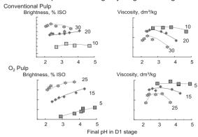
Figure 10.17. The influence of the bleaching conditions on the D1-stage. The chemical charges in kg active chlorine/ton are given in the figures to the left. (Eka Chemicals).
