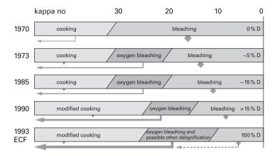
**Figure 14.3.** The development of methods used for delignification and bleaching of kraft pulp. Oxygen bleaching and modified cooking has made it possible to exclude the use of chlorine gas and, in some cases, also of chlorine dioxide. "% D" is the ClO<sub>2</sub>-share of the total amount of oxidation equivalents (ClO<sub>2</sub> and Cl<sub>2</sub>) charged in the first bleaching stage.
