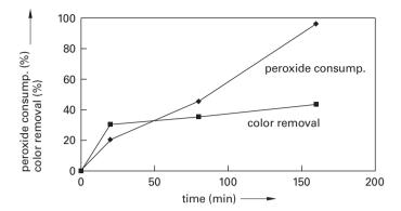
**Figure 9.21.** Alkaline hydrogen peroxide oxidation of residual lignin isolated from kraft pulp after the O-stage showing the gradual consumption of peroxide and the fast removal of color. Oxidation at 50 °C during 160 min (Gärtner 1998).
