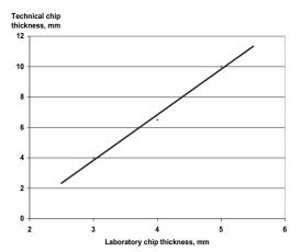
**Figure 16.18.** Kraft cooks with conditions resulting in a shives content of 1 % have been performed on laboratory and technically prepared chips. Shives are intact, undelignified fibre bundles, usually originating from the core of the chip due to insufficient impregnation.
