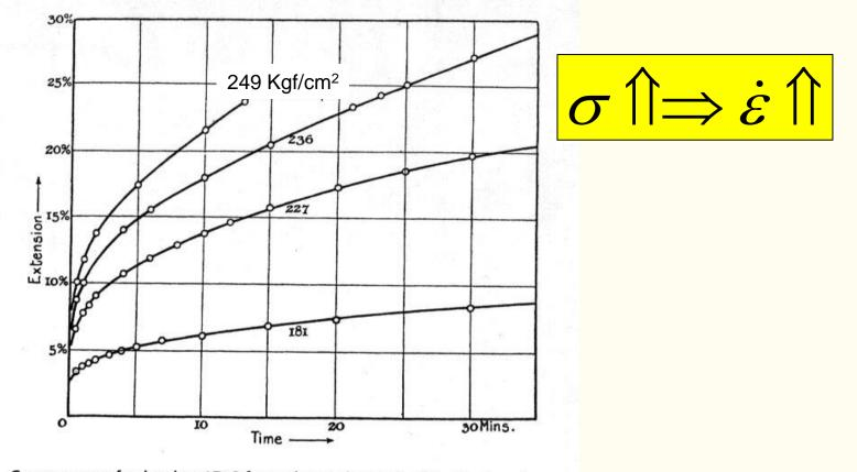
Creep curves for lead at  $17^{\circ}$ C from the early work of Andrade, where  $1 \text{ kg/cm}^2 = 0.0981 \text{ MPa}$ . (From [Andrade 14]; used with permission.)
