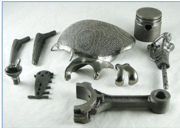
Figure 2. EBM fabricated Ti6Al4 V biomedical and mechanical components.
