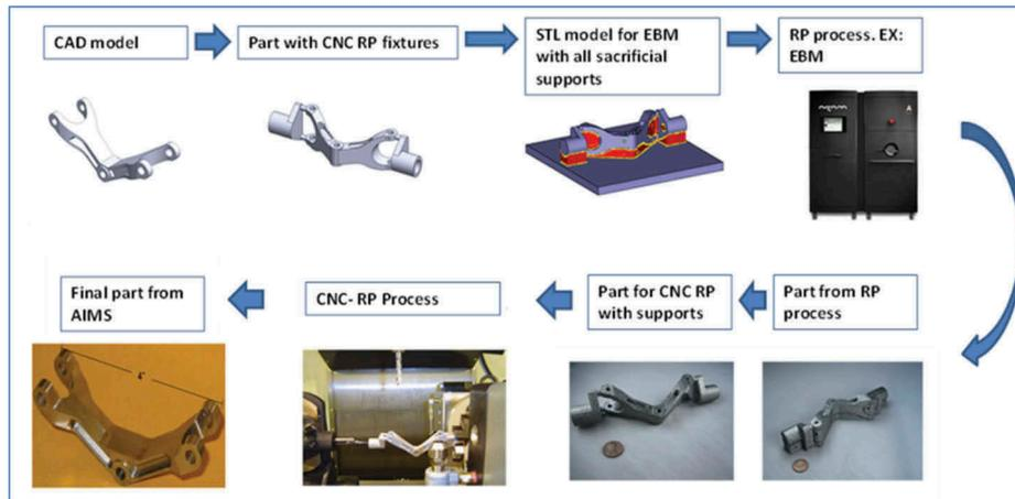
Figure 1. AIMS: Integrated AM and CNC-RP integrated flow illustration.
