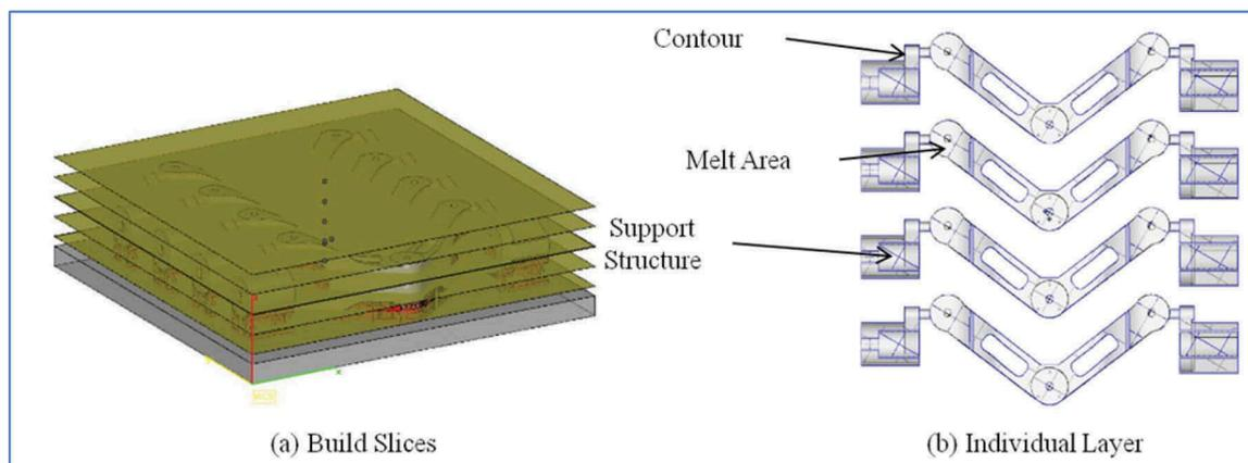
Figure 4. (a) Schematics of EBM build slices and (b) Individual layer showing the support and melt features for the sample part in this study.
