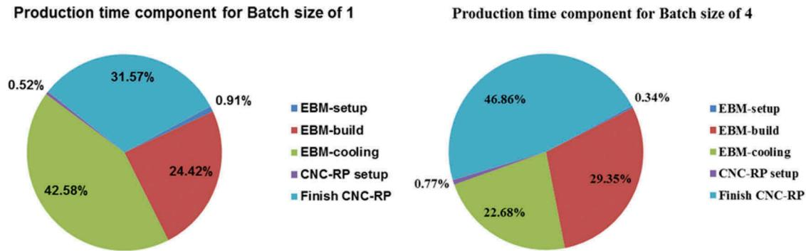
Figure 6. Time components in the AIMS production based on batch size for sample part.
