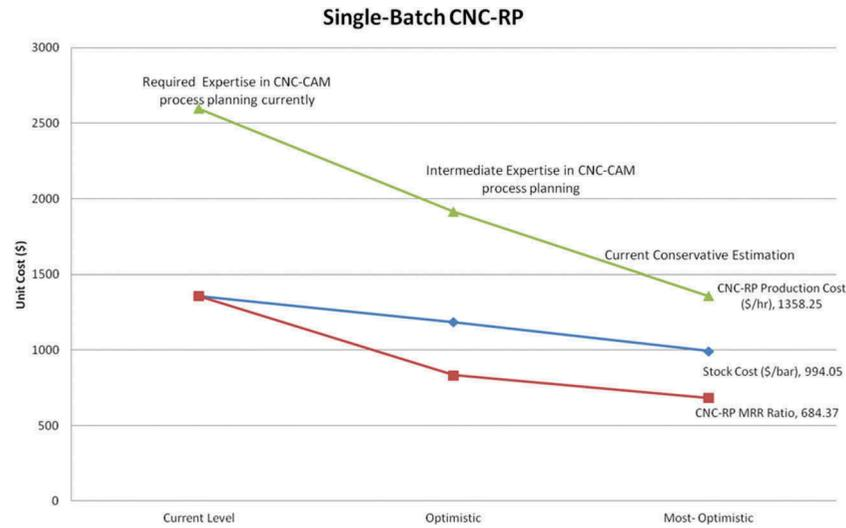
Figure 8. Influences of cost-factors on single-batch production through CNC-RP for sample part.
