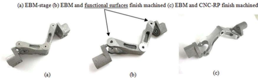
Figure 10. Functional surfaces and CNC-RP finish machining.
