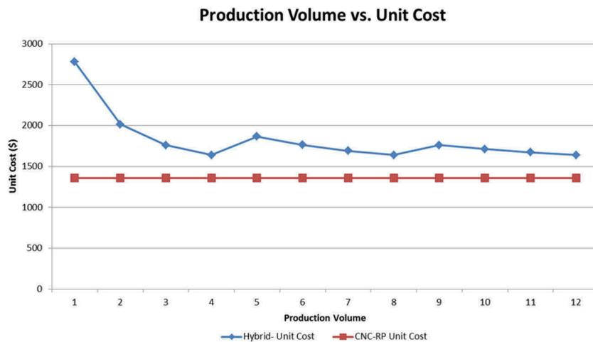
Figure 5 Unit cost through batch production in CNC-RP and hybrid process AIMS for the sample part.
