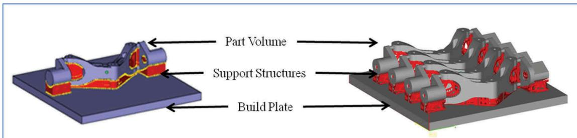
Figure 3. Unit and batch production of sample part in EBM with sacrificial supports for the subtractive stage.
