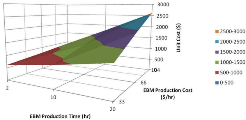
Figure 9. Influences of EBM production time and cost on single-batch production through AIMS.
