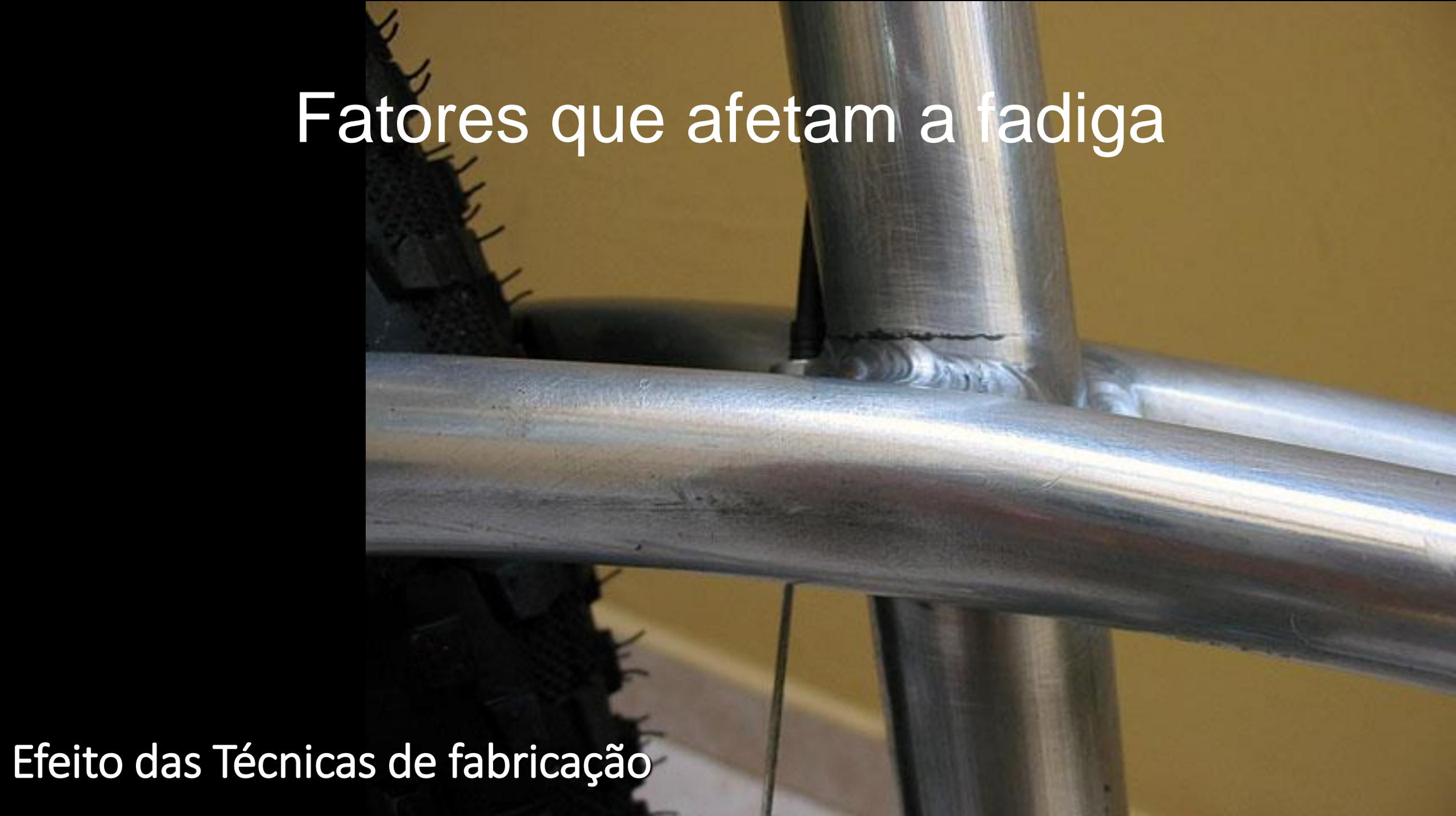
A close-up photograph of a metal bicycle frame joint. The frame consists of several cylindrical tubes. A prominent weld joint is visible where a vertical tube meets a horizontal tube. A small, dark crack is clearly visible at the top of the weld joint. The background is a plain, light-colored wall. The image is used to illustrate factors affecting fatigue in metal structures.
