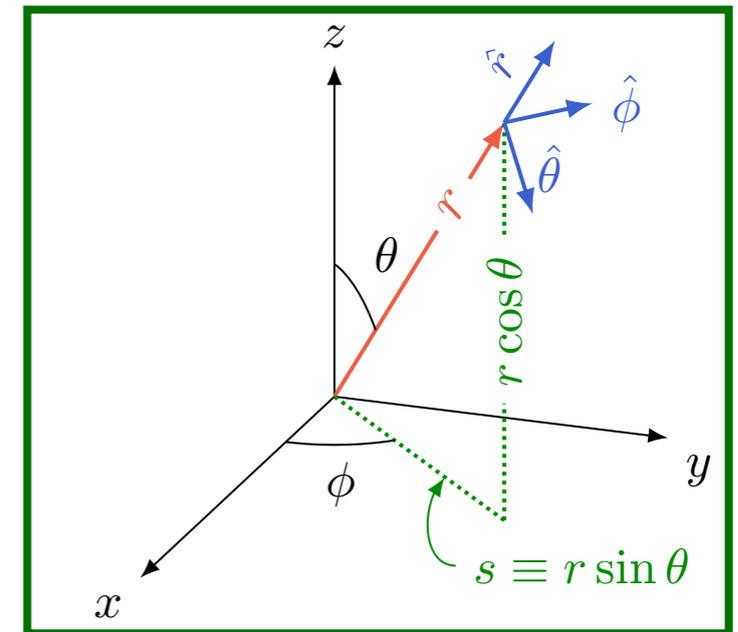
$$\vec{\nabla} \cdot \vec{v} = \frac{1}{r^2} \frac{\partial (r^2 v_r)}{\partial r} + \frac{1}{r \sin \theta} \frac{\partial (\sin \theta v_\theta)}{\partial \theta} + \frac{1}{r \sin \theta} \frac{\partial v_\phi}{\partial \phi}$$
