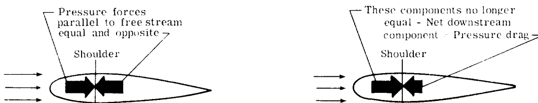
(b) Ideal fluid airfoil (no pressure drag).
