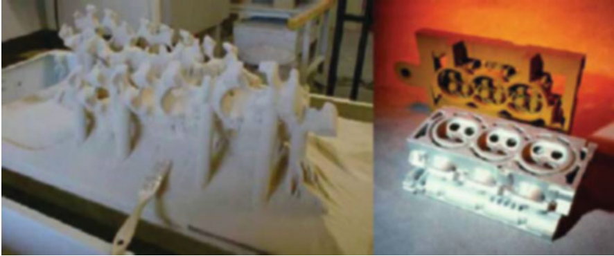
Fig. 14.12 Sand casting pattern for a cylinder head of a V6, 24-valve car engine ( left ) during loose powder removal and ( right ) pattern prepared for casting alongside a finished casting (Joint project between CAD/CAM Becker GmbH and VAW Südalumin GmbH, made on an EOSINT S laser-sintering machine, courtesy EOS)
