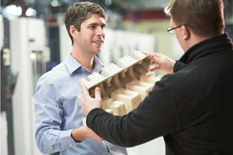
Fig. 18.7 A paper pulp molding tool shown with a molded packaging component (Courtesy of RedEye Redeyeondemand.com)
