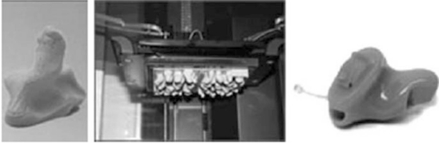
Fig. 2.9 RM of custom hearing aids, from a wax ear impression, on to the machine to the final product (photo courtesy of Phonak)
