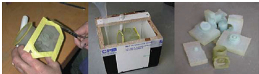
Fig. 14.13 RTV molding process steps (Courtesy MTT Technologies Group)
