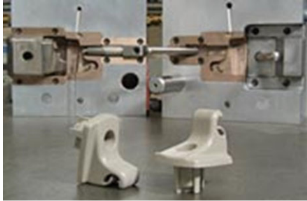
Fig. 18.4 A direct metal laser sintered tool set, with two parts that have been molded from them
