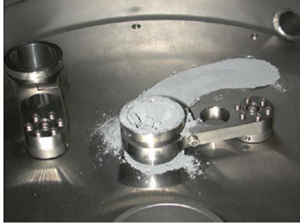
Fig. 5.14 3D Micromac Powder Feed System. In this picture, only one of the powder feeders (located over the build cylinder) is filled with powder (courtesy: Laserinstitut Mittelsachsen e.V.)
