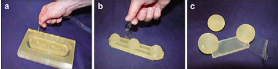
Fig. 9.2 Support material removal for three golf balls made using a Solidimension machine, showing: (a) the balls still encased in a central region, being separated from the larger block of bonded material; (b) the support material is glued in an accordion-like manner so that the excess material can be pulled out easily as a continuous piece; and (c) the balls after complete removal of excess support material (Courtesy 3D Systems)
