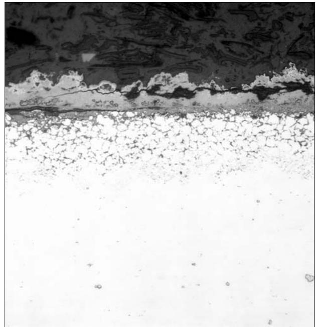
Figure 53 - Intergranular oxidation. (200X)
