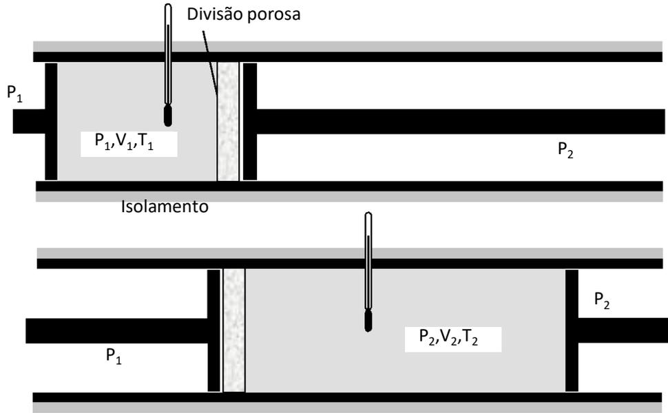
$$w_1 = - \int_{V_1}^0 P dV = -P_1 \int_{V_1}^0 dV = P_1 V_1$$
