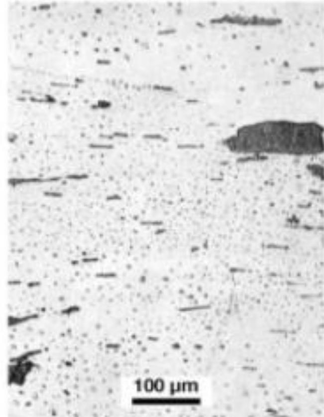
**Fig. 5.10** Drying marks. The small spots are drying marks from water droplets. Material is "rough iron" (See "Historical Direct Reduction Products" section of Chapter 2, "Processes in Steel Production," in this book) with many large non-metallic inclusions.
