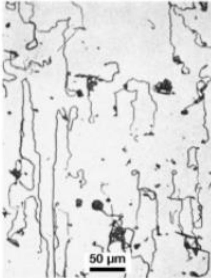
**Fig. 5.9** Filiform (filament-shaped) rusting that can occur during improper sample storage after polishing.
